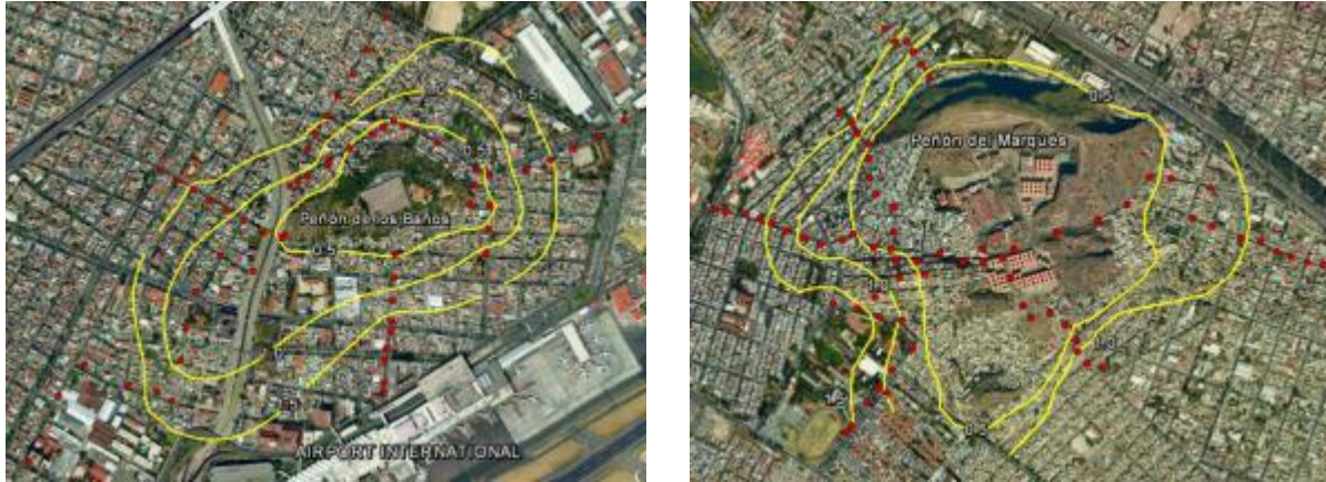
Figure 2.3. Yellow lines give the zonation for Peñón de los Baños (left) and Peñón del Marqués (right). Red dots indicate measurement points. Values in contours correspond to period in seconds.
