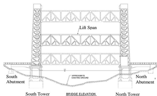
**Figure 1.2.** Fruitvale Railroad Bridge, Elevation View
