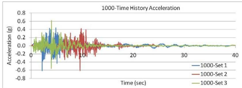
**Figure 2.6.** Spectrum-Compatible Time Histories for Vertical Components (1000-year)
