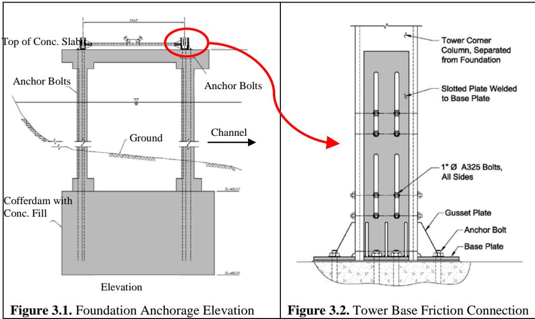
**Figure 3.1.** Foundation Anchorage Elevation
