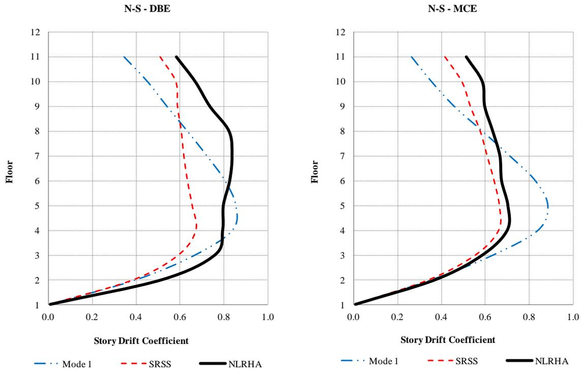
**Figure 4.2.** North south direction story drift coefficients
