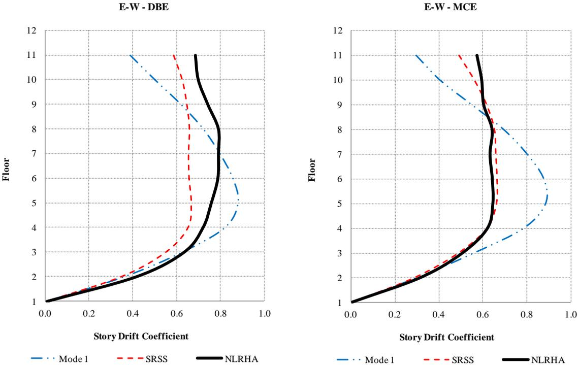
Figure 4.1. East west direction story drift coefficients
