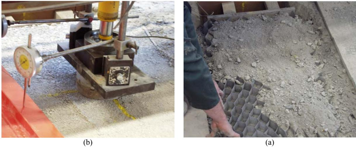
**Figure 3.** Test installations (a) Geocell installation beneath the footing, and (b) Loading plate located in centreline of the trench
