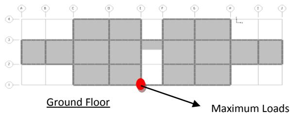
**Figure 4.** Plan of the Building showing the Column bearing the maximum Loads.
