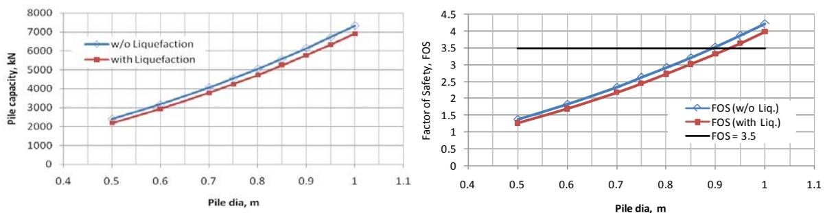
**Figure 7.** Variation of Pile Capacity (kN) and Factor of safety with the Pile diameter (m) with and without Liquefaction
