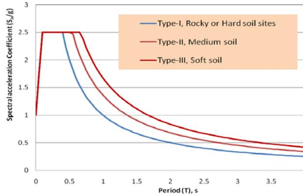
**Figure 2.** Response Spectra for Rock and Soil sites as per IS 1893 for five percent Damping
