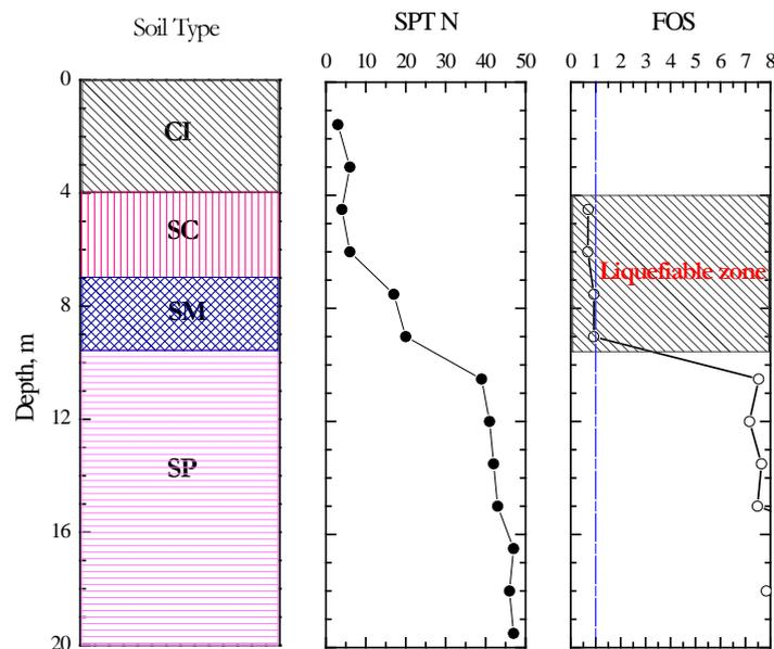
**Figure. 6** Typical soil profile data considered and its liquefaction susceptibility
