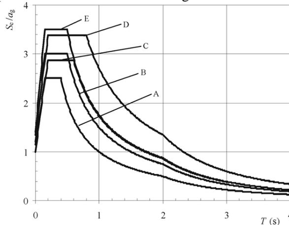
**Figure 3.** Elastic Response Spectra (Type I) for Ground Types A to E for five percent Damping (EN 1998).
