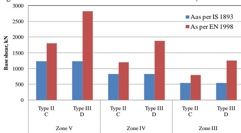
**Figure 5.** A bar chart comparing the base shear forces as per the two codes
