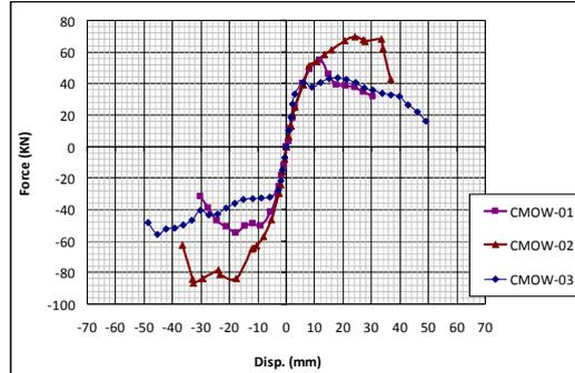
**Figure 12.** The envelopes of hysteresis curves of CMOW specimens
