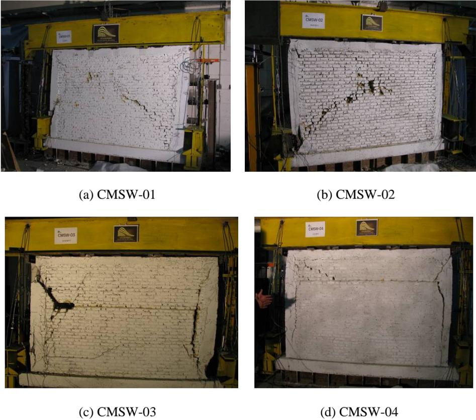
**Figure 9.** Cracking patterns of the wall specimens
