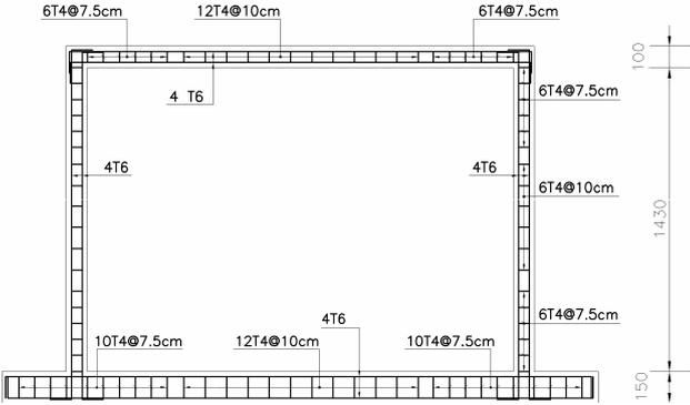
**Figure 3.** Reinforcement details of the wall specimens (dimensions in mm)
