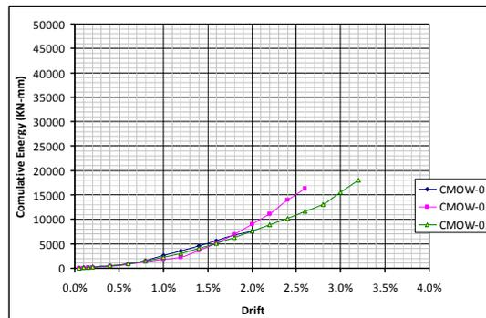
**Figure 13.** Cumulative energy dissipation of CMOW specimens
