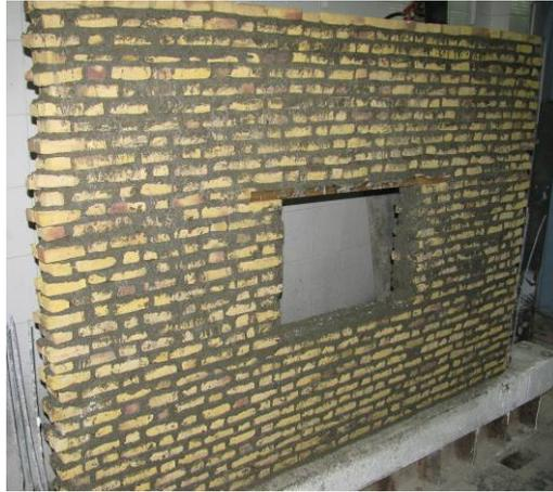
**Figure 5.** CMOW-01 and CMOW-03 with 80 cm length lintel
