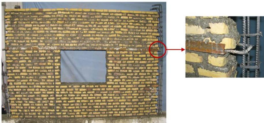
**Figure 6.** CMOW-02 with lintel band and its connection to the vertical tie
