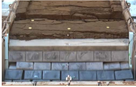
Photo3 Collapsed final situation of Case3 (Max. 818gals)
