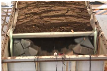
Photo2 Collapsed final situation of Case1 (Max. 1000gals)
