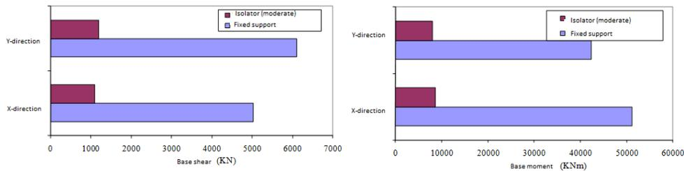
Figure 3.14 Base shear forces and base flexural moments for both the original structure and the base isolated structure
