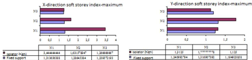
**Figure 3.20** Maximum soft storey index in both X and Y directions for both the original structure and the base isolated structure
