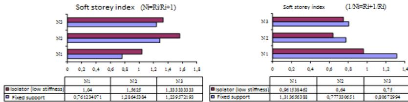
**Figure 3.4** Soft storey index in X direction for both the original structure and the base isolated structure
