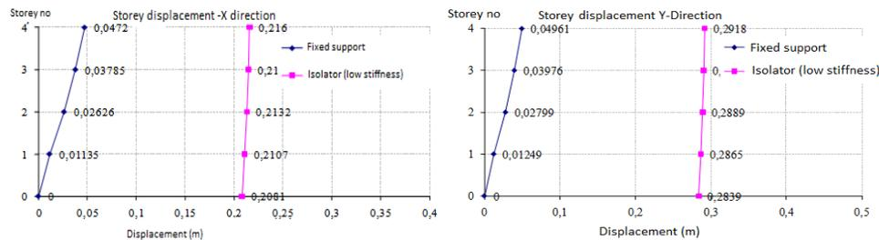
**Figure 3.1** Storey displacements in both X and Y directions for both the original and the base isolated structures
