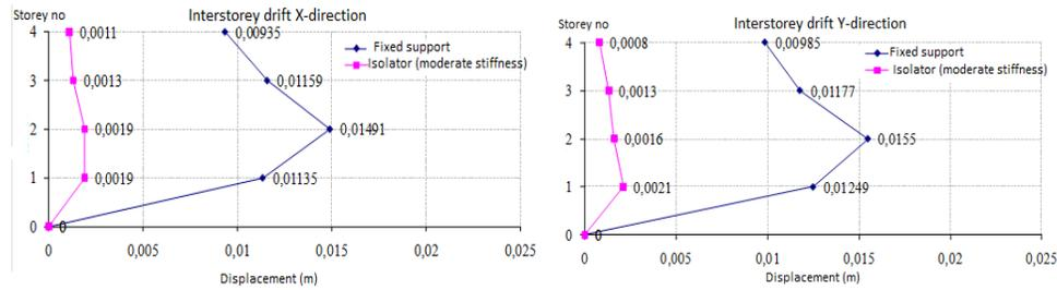
**Figure 3.9** Interstorey drifts in both X and Y directions for both the original and the base isolated structures
