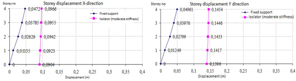
**Figure 3.8** Storey displacements in both X and Y directions for both the original and the base isolated structures
