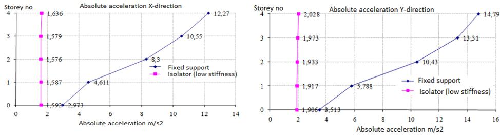
**Figure 3.3** Absolute storey accelerations in both X and Y directions for both the original and the base isolated structures
