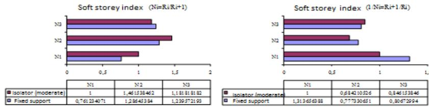
Figure 3.11 Soft storey index in X direction for both the original structure and the base isolated structure
