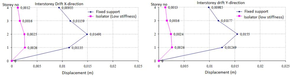
**Figure 3.2** Interstorey displacements in both X and Y directions for both the original and the base isolated structures
