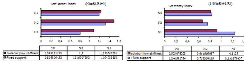
**Figure 3.5** Soft storey index in Y direction for both the original structure and the base isolated structure
