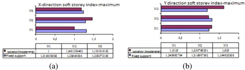
Figure 3.13 Maximum soft storey index in both X and Y directions for both the original structure and the base isolated structure
