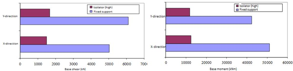
**Figure 3.21** Base shear forces and base flexural moments for both the original structure and the base isolated structure
