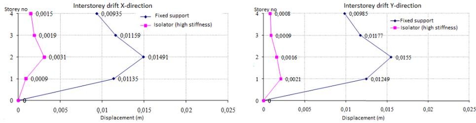
**Figure 3.16** Interstorey displacements in both X and Y directions for both the original and the base isolated structures
