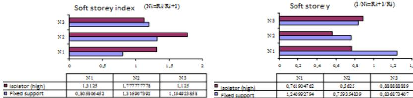
**Figure 3.19** Soft storey index in Y direction for both the original structure and the base isolated structure
