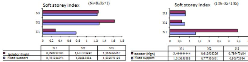
**Figure 3.18** Soft storey index in X direction for both the original structure and the base isolated structure
