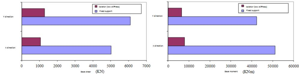
**Figure 3.7** Base shear forces and base flexural moments for both the original structure and the base isolated structure
