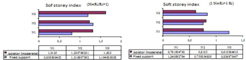
Figure 3.12 Soft storey index in Y direction for both the original structure and the base isolated structure
