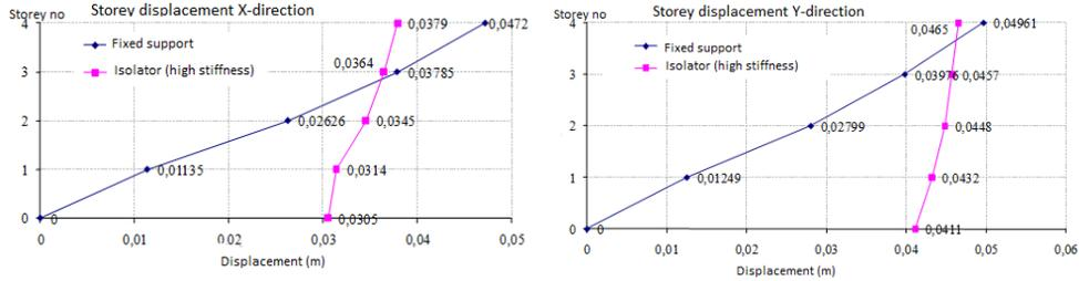
**Figure 3.15** Storey displacements in both X and Y directions for both the original and the base isolated structures
