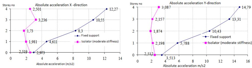
**Figure 3.10** Absolute storey accelerations in both X and Y directions for both the original and the base isolated structures
