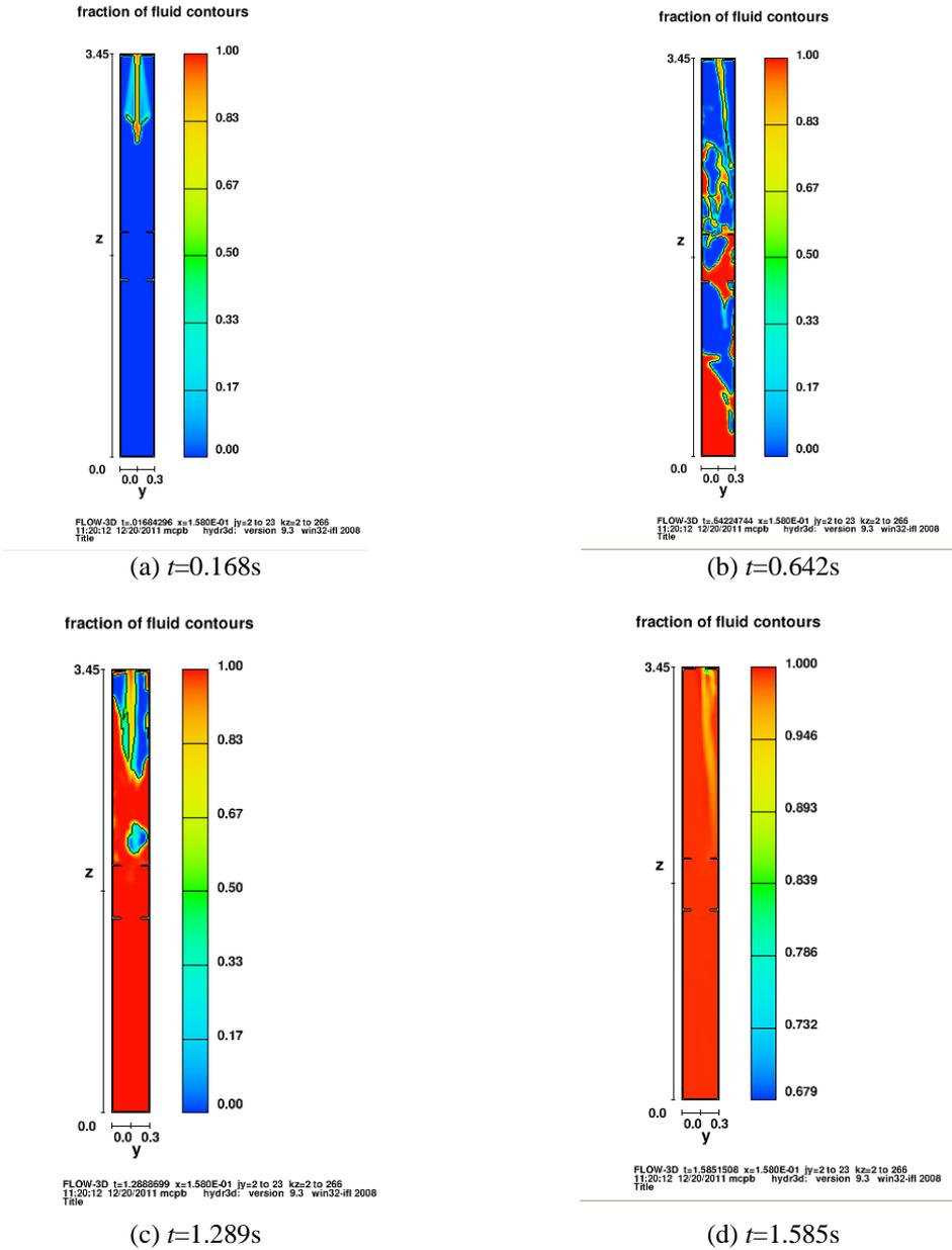
**Figure 3.1.** Fraction of concrete at different time on x-z plane
