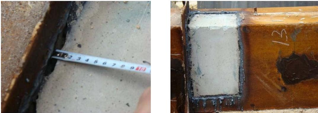
**Figure 4.1.** The shrinkage below the clapboard of the tube
