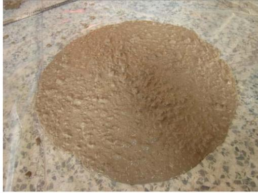
**Figure 2.6.** The Slump test
