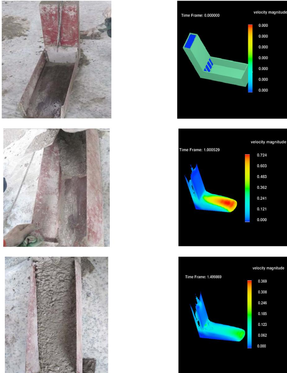
**Figure 2.1** Process of L-Box test in Spatial Space
