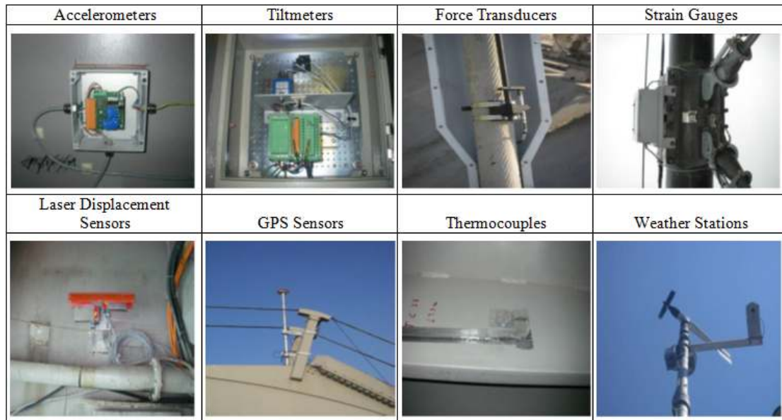
Figure 3. The pictures of the sensors used in the SHM system at the Bogazici Suspension Bridge
