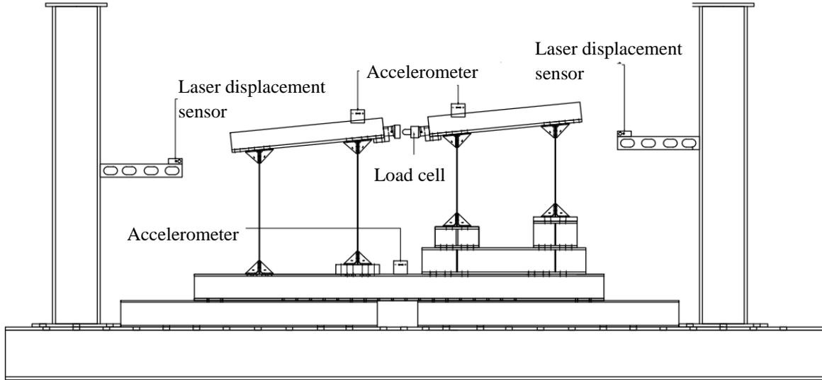
Figure 1. Test models with inclined decks and sensors
