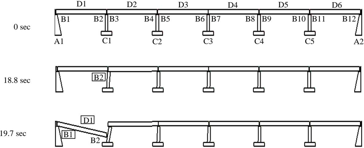
Figure 7. Failure process of the bridge with level decks under 200% of the JR Takatori record.
