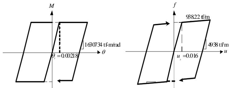
Figure 5. Material property (a) column (b) isolator
