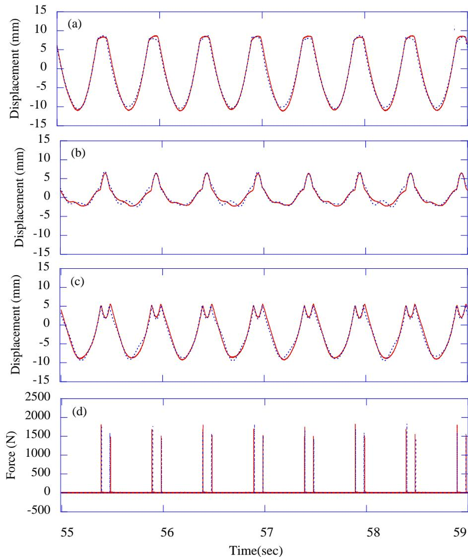
Figure 3. Comparison of numerical simulation (dashed curve) and experimental data (solid curve) : (a) displacement of the left bridge (b) displacement of the right bridge (c) relative displacement between two bridges (d) pounding force
