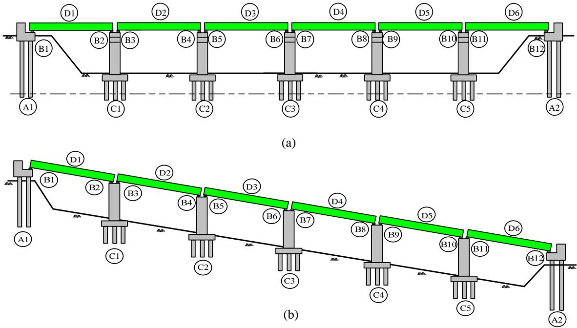
Figure 4 Target bridges with (a) level decks (b) inclined decks
