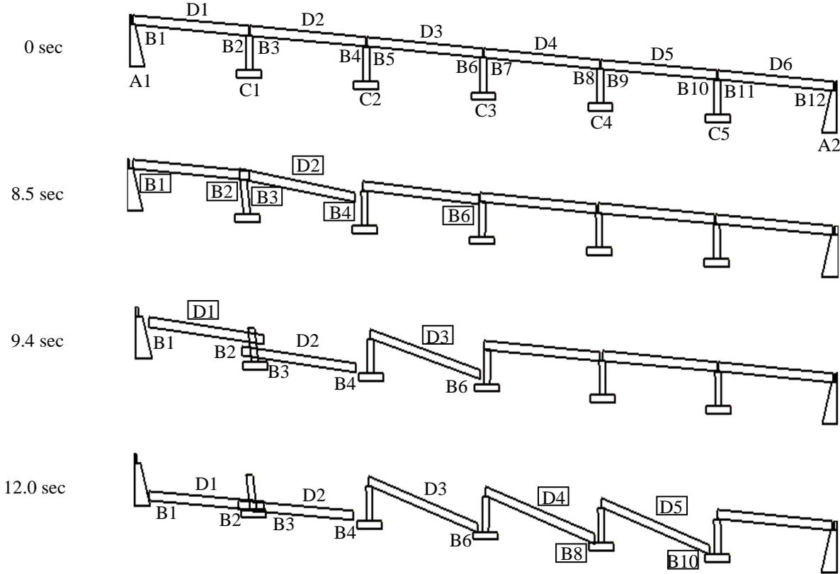
Figure 8. Failure process of the bridge with 8% inclined decks under 200% of the JR Takatori record.
