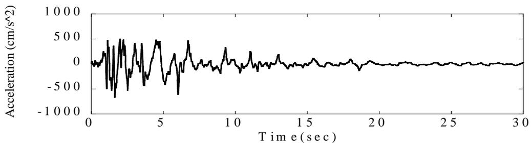
Figure 6. Ground motion recorded at JR-Takatori station in the 1995 Kobe earthquake
