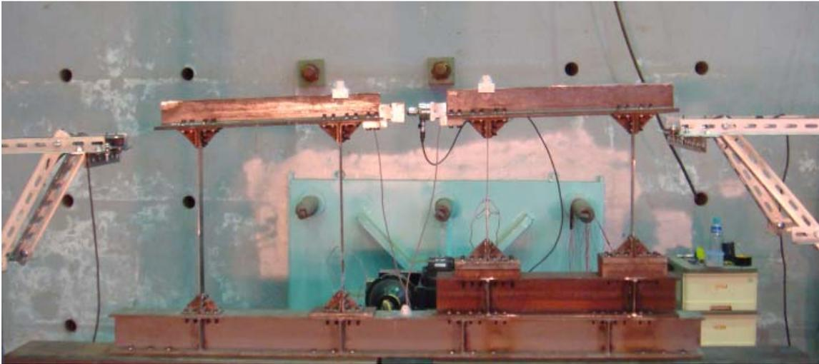
Figure 2. Photo of the test models and sensors installed on a shaking table
