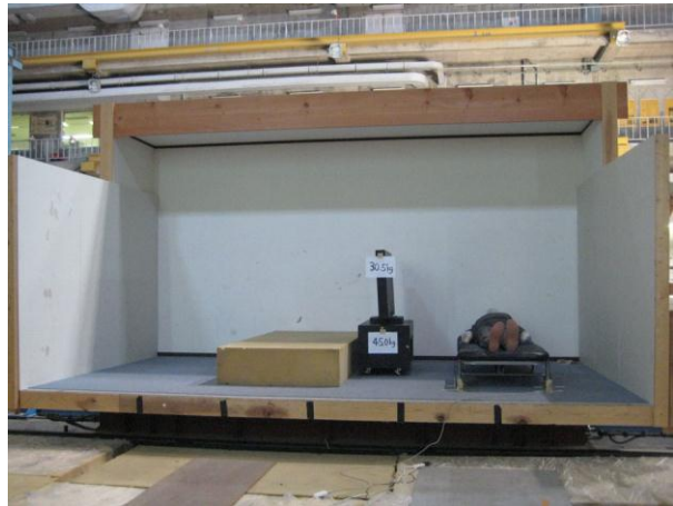
Photo 2. One scene of television turnover test.
