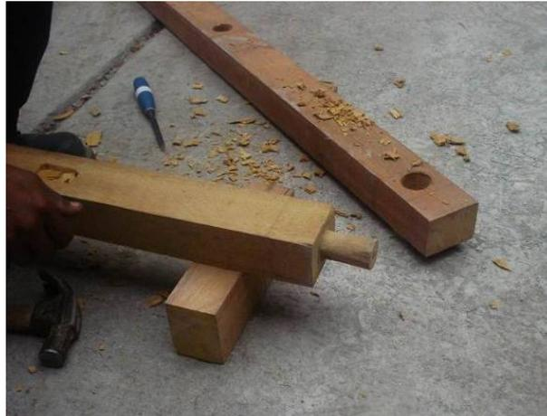
**Figure 2.** Typical mortise and tenon joint.
