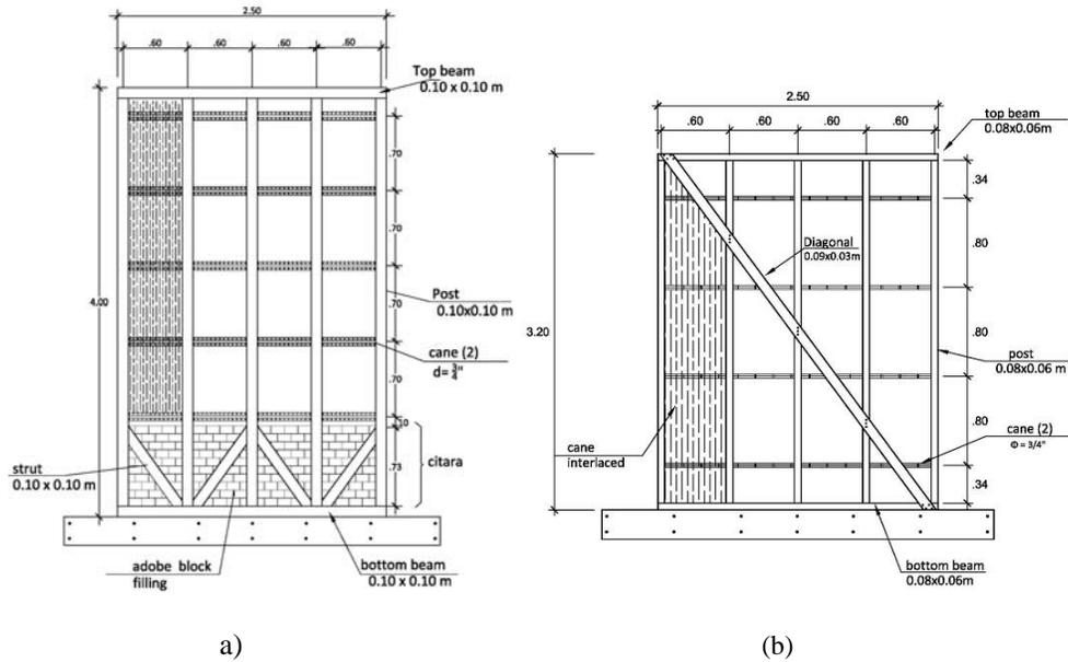
**Figure 1.** Quincha wall specimens: (a) with “citara”; (b) with diagonal.
