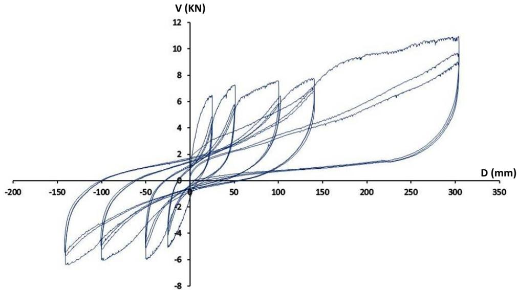
Figure 3. Load – displacement curve. MA2.
