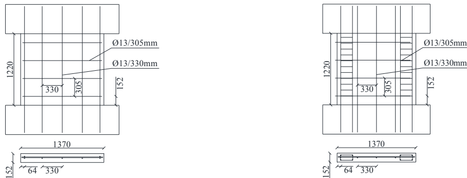
Figure 2.1. Steel reinforcement of RC wall a) tested by (Orakcal et al. 2009) b) ductile wall (measures in mm).
