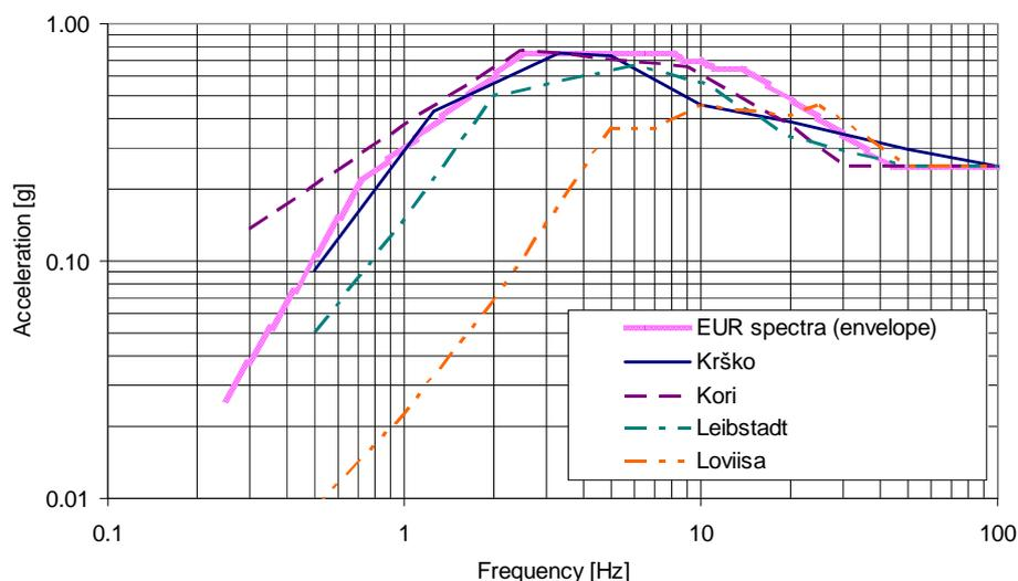
**Figure 4.** Spectral shapes of median uniform hazard spectra in the literature
