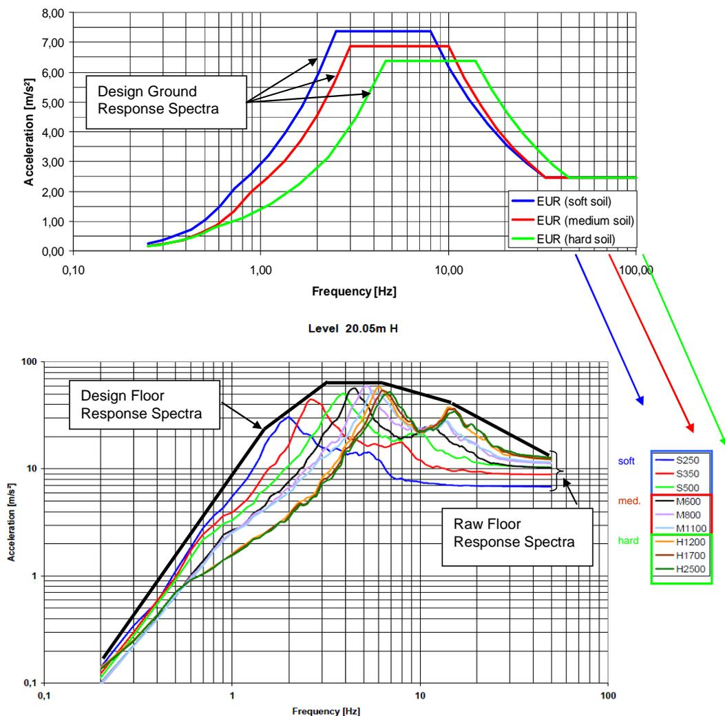
**Figure 3.** Generation of design floor response spectra in the KERENA seismic design
