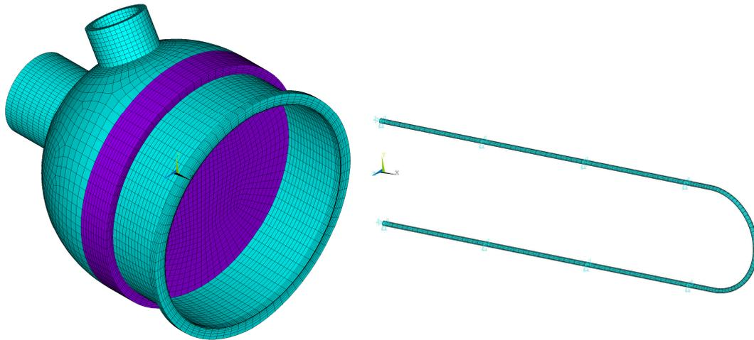
**Figure 5.** Finite element model of emergency condenser wall (left) and tube (right)
