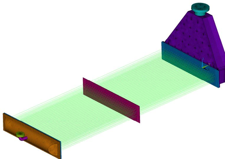
**Figure 6.** Finite element model of the containment cooling condenser
