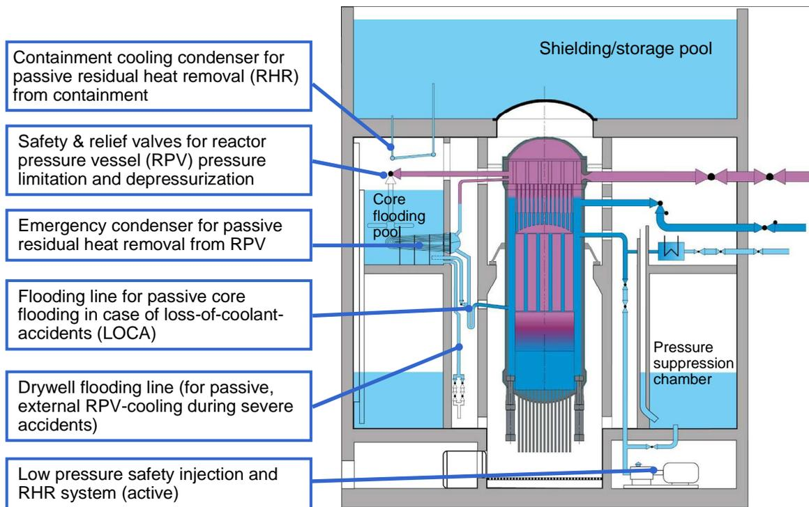
**Figure 2.** Schematic drawing of the KERENA BWR indicating key safety functions
