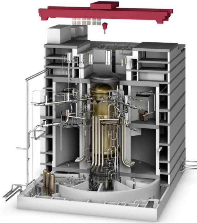
**Figure 1.** Reactor building of the KERENA BWR
