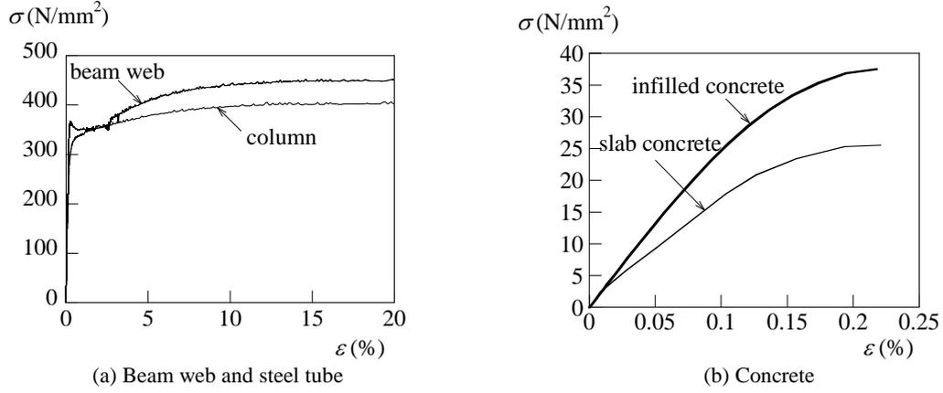
**Figure 2.** Relation of stress-to-strain ratio (example)
