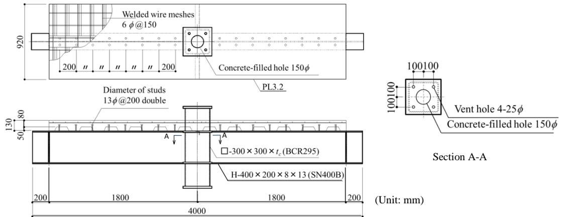
**Figure 1.** Specimen (CFT column)**Table 3.** Results of tensile test
