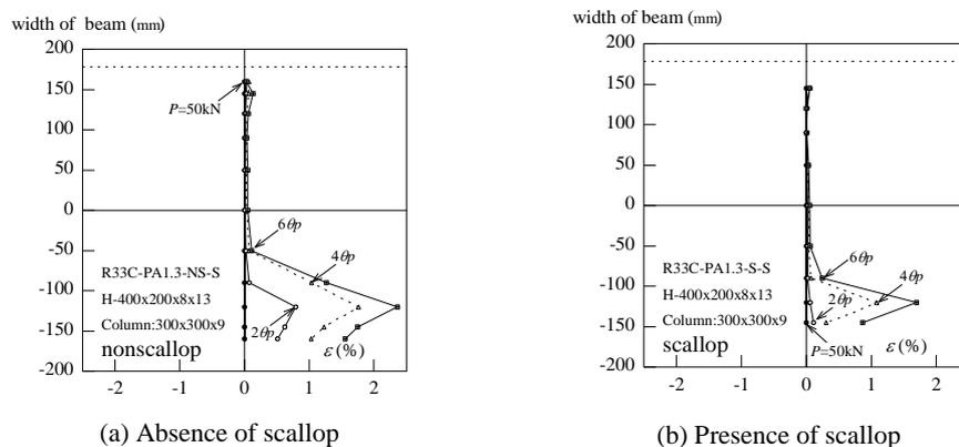
**Figure 7.** The distribution of strain at beam web
