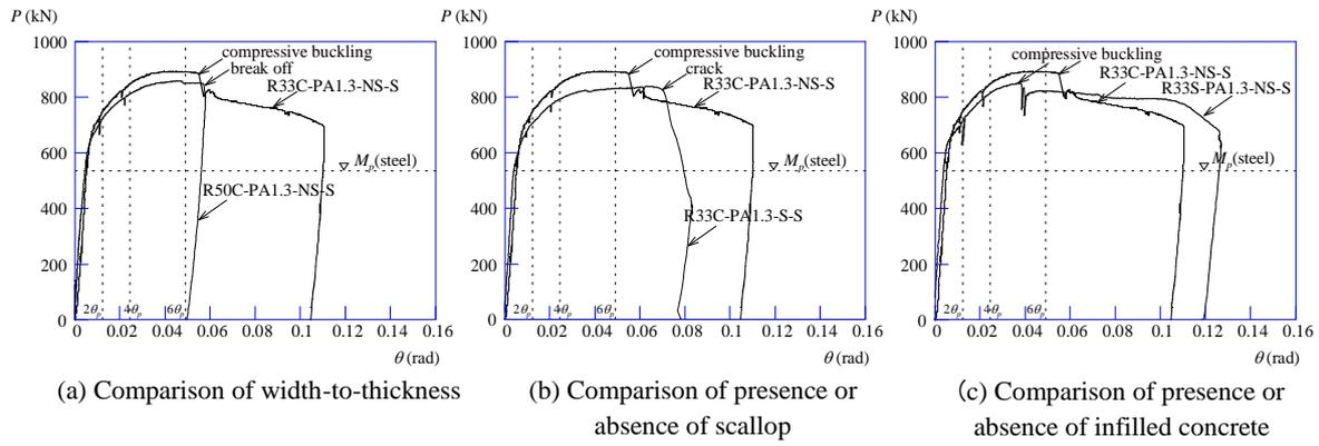
**Figure 6.** Relation between load  $P$  and slope angle of beam  $\theta$
