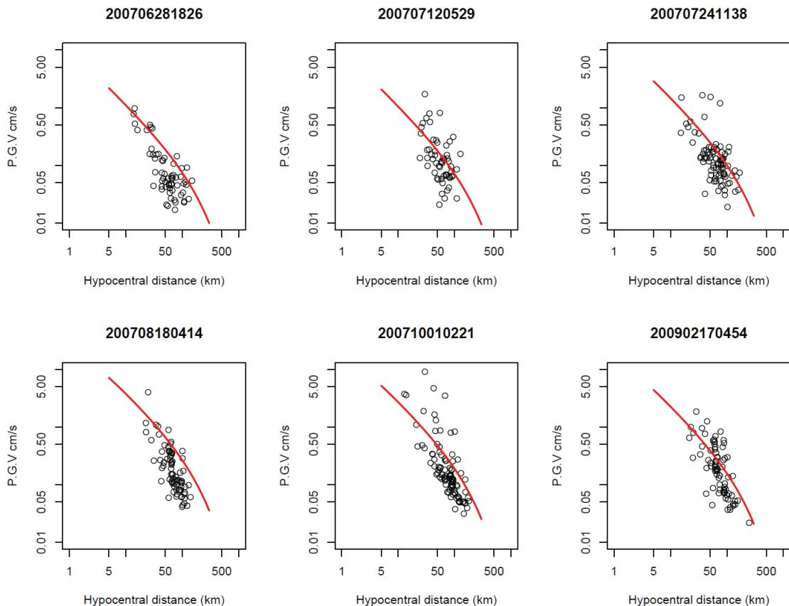
**Figure 2.** Comparison of observed PGVs and predictions by Si and Midorikawa (1999).
