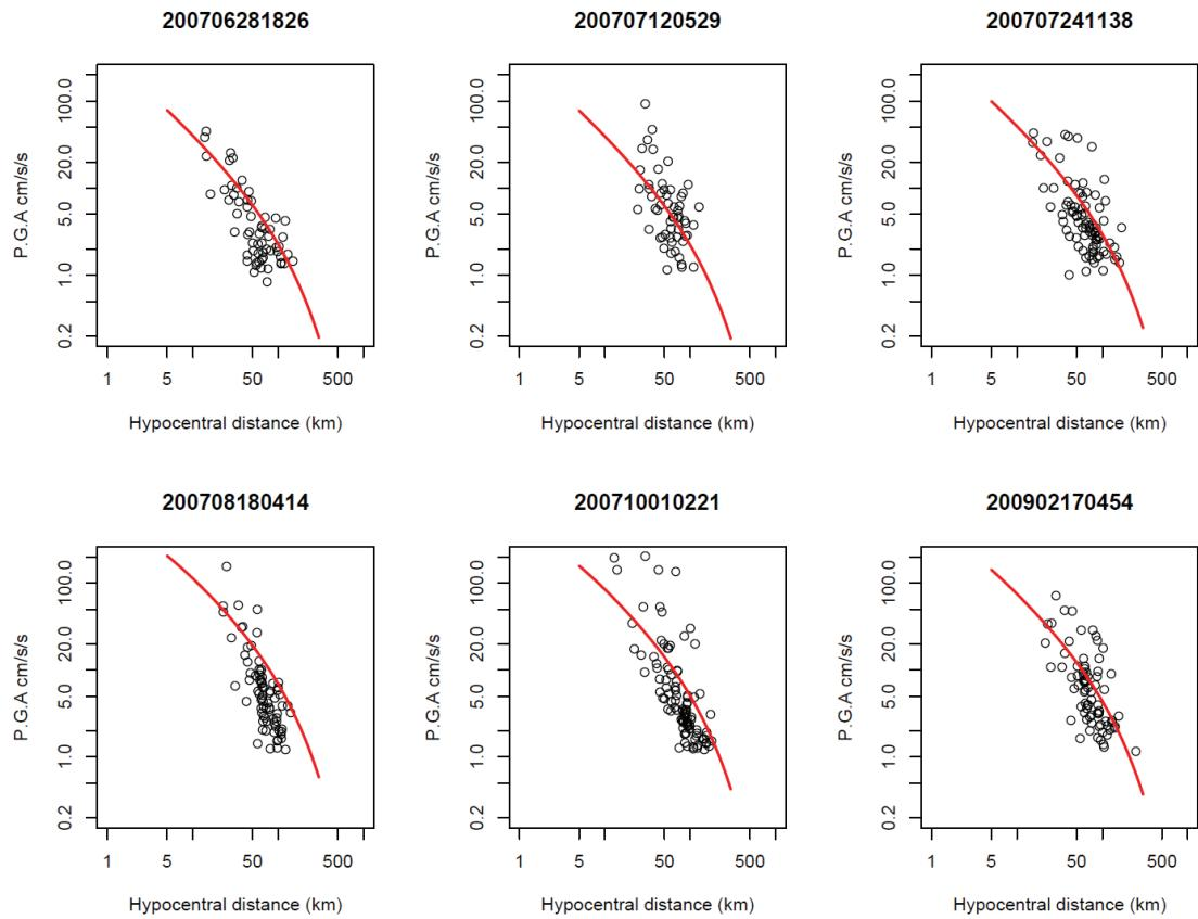
**Figure 1.** Comparison of observed PGAs and predictions by Si and Midorikawa (1999).
