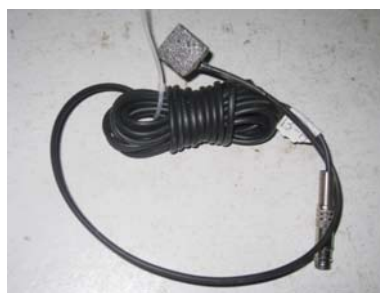
Figure 2.1. SA with embedded PZT patch and wire Figure 2.2. Cross section of the CFST specimen
