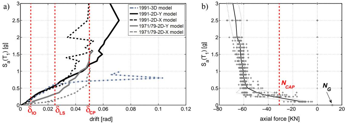
**Figure 5.** (a) Median of global drift ratios for “non-collapse” cases and capacity limits corresponding to different limit states; (b) local force demand in one member and corresponding axial force capacity,  $N_{CAP}$ .
