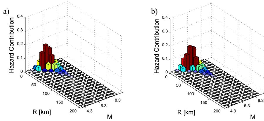
**Figure 3.** Seismic hazard disaggregation of  $S_a(T_1)$ , for  $T_1 = 1.0$  s (a) and 1.6 s (b), for 475 yrs return period.
