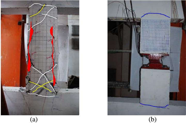
Figure 5.3 Damage distribution: (a) Traditional RC coupling beam; (b) Hybrid coupling beam
