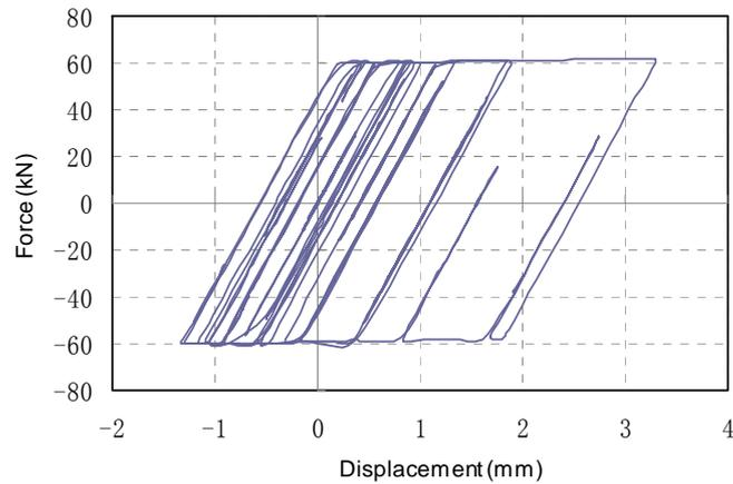
**Figure 6.4** Hysteretic curve of a typical damper
