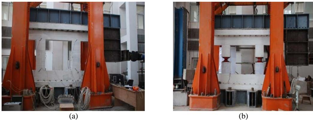
**Figure 4.2** Specimens under loading frame: (a) Traditional RC coupling beam; (b) Hybrid coupling beam
