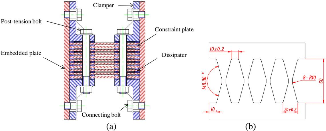
**Figure 3.1** Metallic damper: (a) Assembling modular damper; (b) Configuration of dissipater
