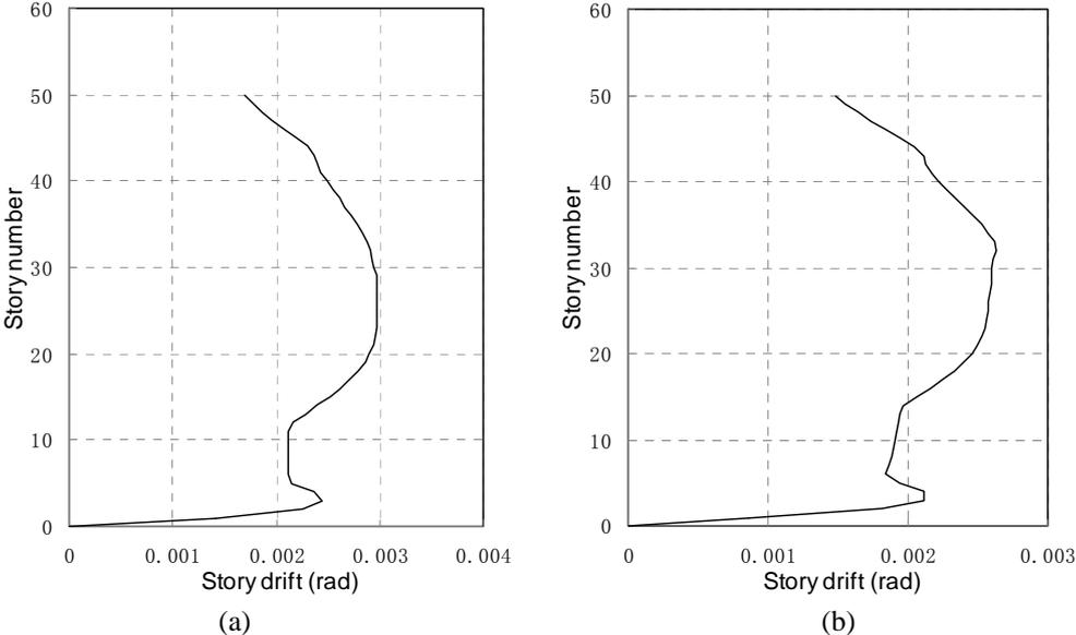
**Figure 6.2** Maximum responses in longitudinal direction: (a) Original structure; (b) Structure with hybrid beams
