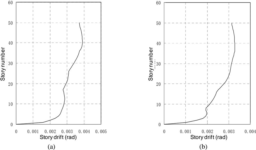
**Figure 6.3** Maximum responses in lateral direction: (a) Original structure; (b) Structure with hybrid beams
