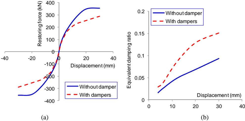
Figure 5.2 Behavior comparison: (a) Skeleton curves; (b) Equivalent damping ratios
