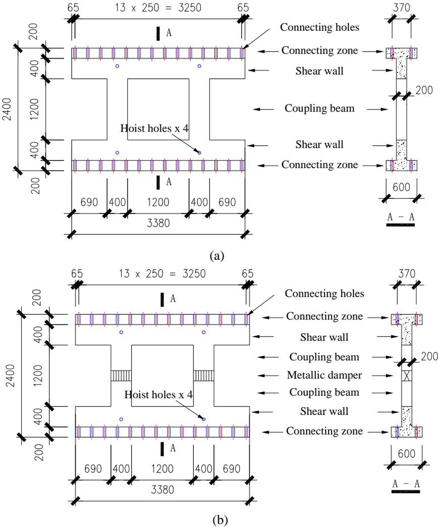
Figure 2.1 Specimens: (a) Traditional coupling beam; (b) Hybrid coupling beam
