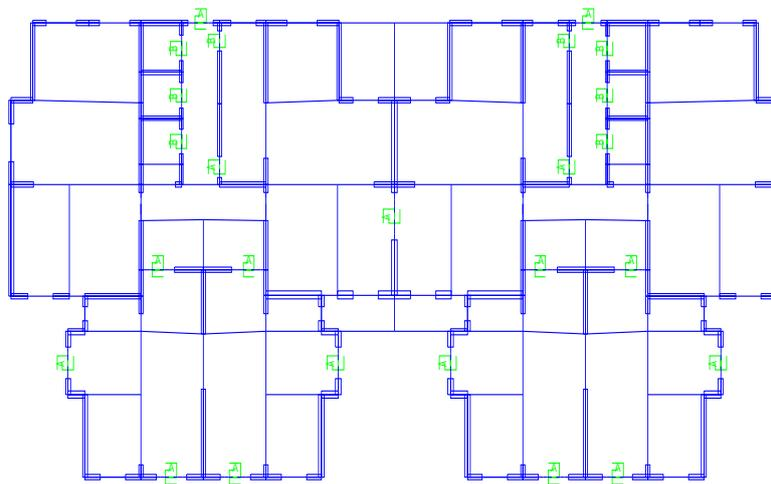
**Figure 6.1** Standard plan view and damper distribution
