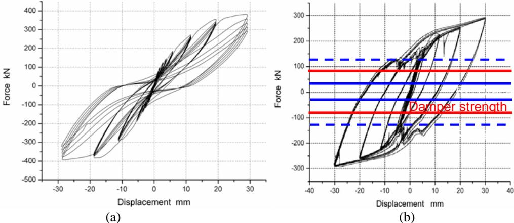
Figure 5.1 Hysteretic curves: (a) Traditional RC coupling beam; (b) Hybrid coupling beam
