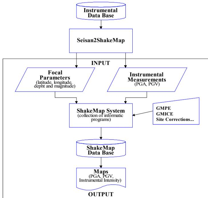
Figure 2.1. Simplified ShakeMap flowchart at IM.
