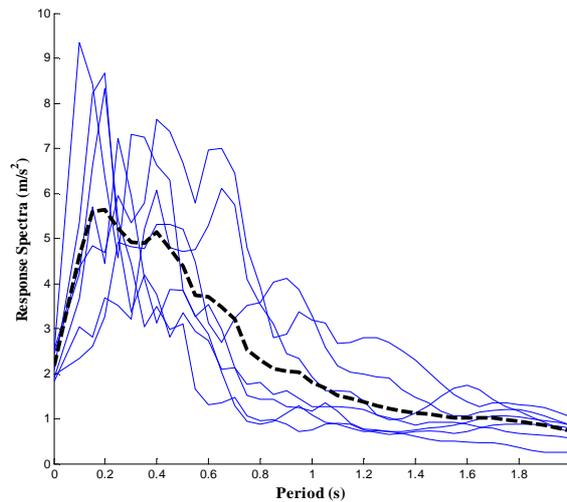
**Figure 2.10.** Elastic response spectra of 7 accelerograms for soil category B and their mean spectra (thick line).
