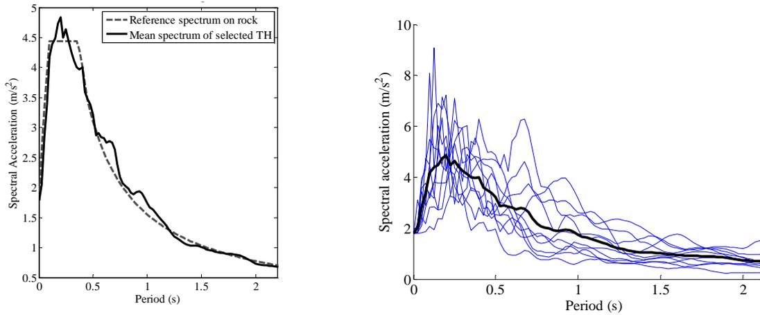
**Figure 2.3** Left: comparison of NTC08 response spectrum for the town of Teramo (dashed line) and the average response spectrum (structural damping 5%) of the selected accelerograms. Right: elastic response spectra of the 10 accelerograms selected, along with their mean spectrum (thick line).
