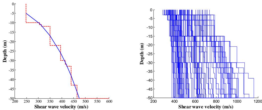
**Figure 2.4.** Example of shear wave velocity profile generated using Monte Carlo simulation (left) and random shear wave velocity profiles obtained using the proposed procedure for a soil category B, with values of  $V_{s,30}$  ranging between 360 and 800 m/s, considering 100 soil profiles (right).
