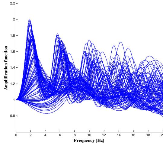
**Figure 2.6.** Amplitude of the transfer function for the soil profiles shown in Figure 2.4 (right)
