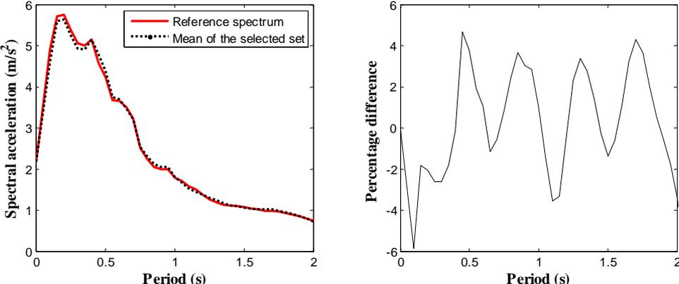
**Figure 2.9.** a) Comparison between the mean spectrum obtained from stochastic ground response analyses and the mean spectrum of the selected set of acceleration time histories to be used for dynamic analysis; b) percentage difference between the two spectra.
