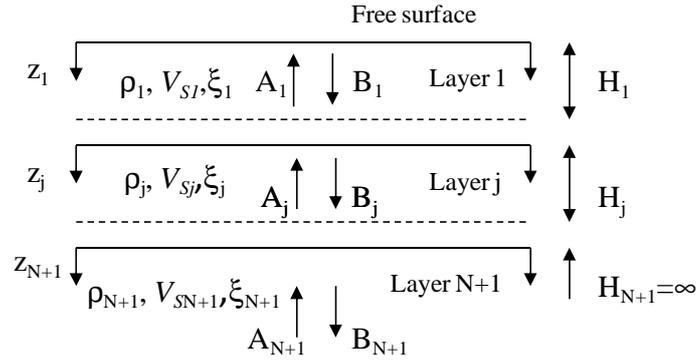
**Figure 2.5.** Viscoelastic layered soil deposit overlaying an elastic bedrock: geometry, geotechnical parameters and amplitudes of the waves traveling upward and downward (modified from Faccioli and Paolucci, 2005)
