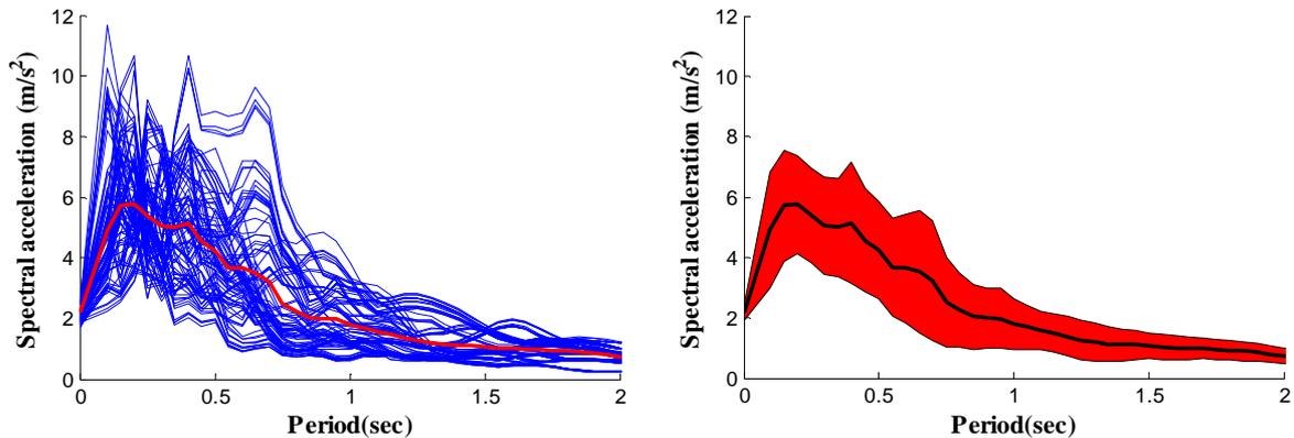
**Figure 2.7.** Left: acceleration response spectra computed for each of the 100 simulations and mean spectrum (thick red line). Right: mean and mean plus/minus one standard deviation (area) acceleration response spectra.
