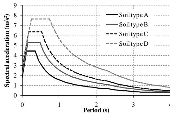
**Figure 2.2** Response spectra for different soil conditions according to NTC08 for Teramo (Central Italy).
