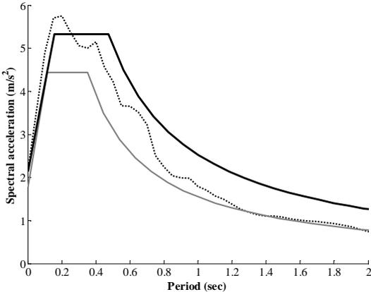
**Figure 2.8.** Comparison of the average response spectrum at the free-surface obtained from site response analyses (dotted line) and the code spectra for type A soil (rock, grey line) and for a type B soil (black thick line).
