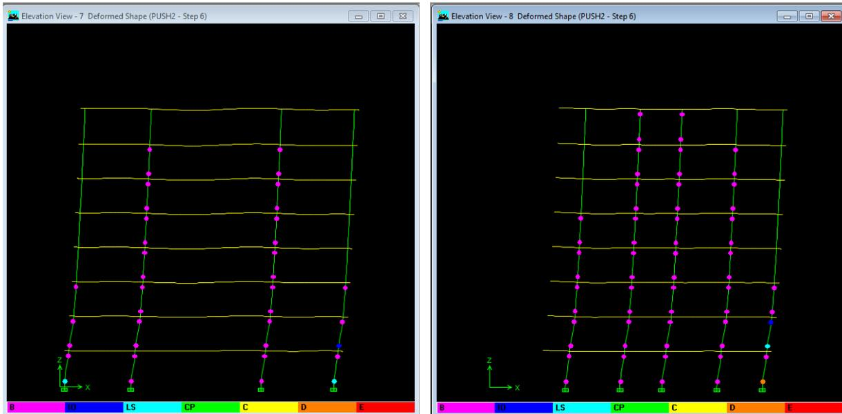
Figure 8. Distribution of the plastic hinges, San Martin tower.
