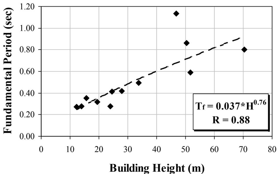
**Figure 7.** Fundamental period of monitored buildings as a function of their height (single values and their regression).
