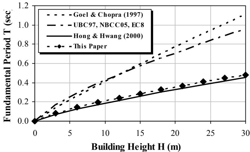
**Figure 8.** Comparison between Code, Goel & Chopra (1997), Hong and Hwang (2000) formulations with the regression obtained from the analysis of Canadian data (this paper).
