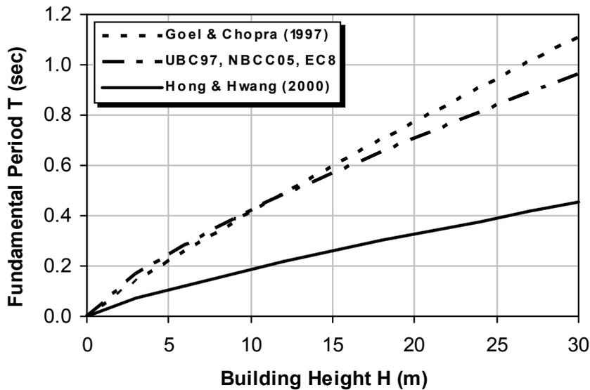
**Figure 2.** Comparison between Code, Goel & Chopra (1997) and Hong & Hwang (2000) formulations of fundamental period of RC buildings.
