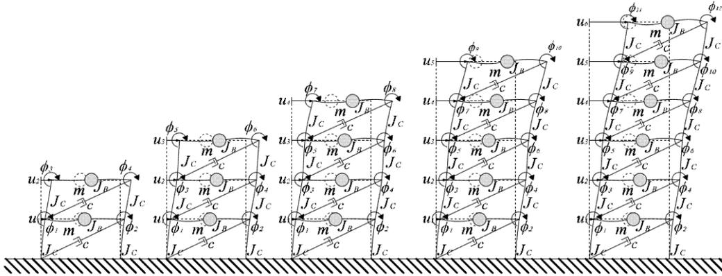
**Figure 5.2.** Schematic representation of the MDOF frame systems used to perform the numerical analysis.
