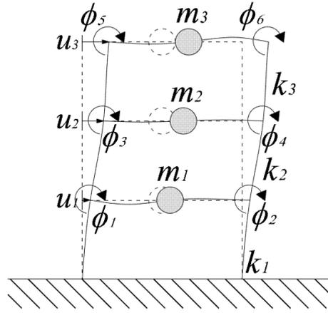
**Figure 3.1.** 3-storey flexible-type structure equipped with interstorey dampers.
