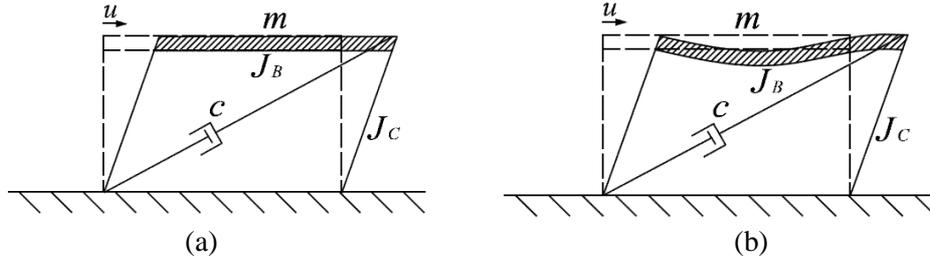
**Figure 5.1.** (a) Shear-type SDOF system equipped with viscous damper; (b) Flexible-type SDOF system equipped with viscous damper.
