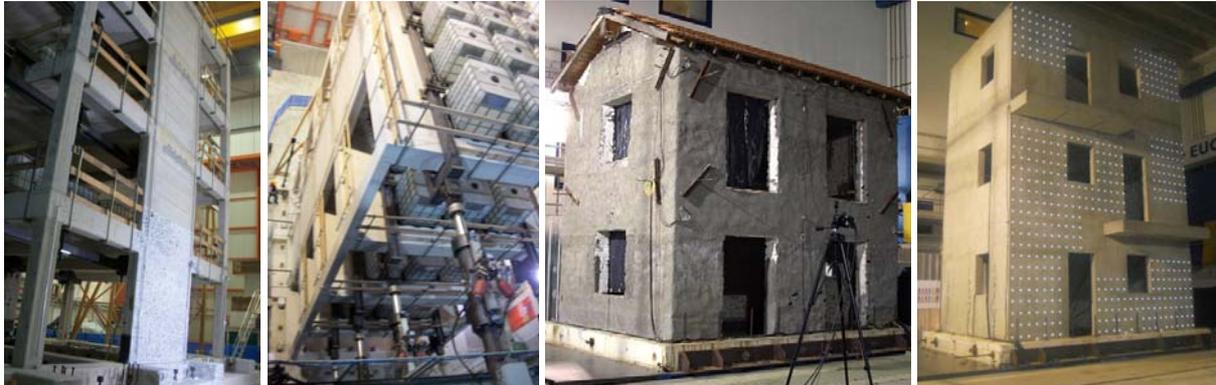
**Figure 4.1.** Views of TA test structures: (a) and (b) SERFIN; (c) "Polyfunctional ...masonry structures" (Peloso et al, 2011); (d) "Seismic ... systems composed of cast-in-situ concrete walls" (Ivorra et al, 2012)
