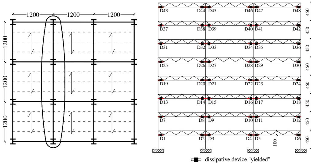
**Figure 3.1.** Analysed structure and numbering of dissipative devices
