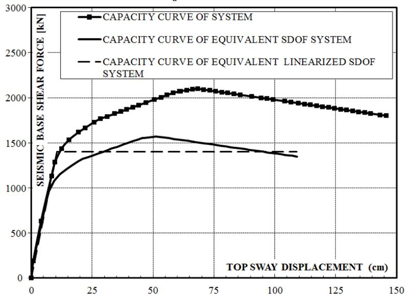
3 BAY – 8 STOREY DTMF  $N_d=665$  kN Second seismic force distribution
