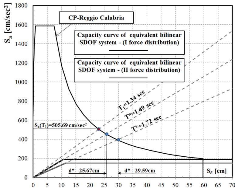
**Figure 4.3.** Application of CSM to the designed DTMF for Reggio Calabria seismic zones
