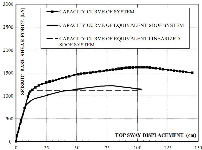
Figure 4.2. Push-over curves and bilinear approximation
