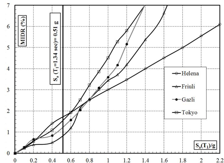
**Figure 5.4.** Maximum Interstorey Drift Ratio versus spectral acceleration
