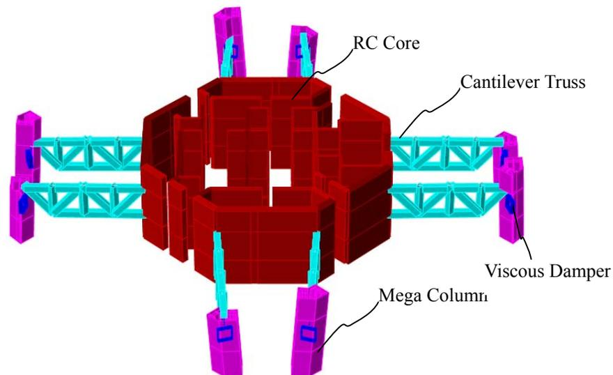
**Figure 3.3** Cantilever Truss Dampers in SAGT
