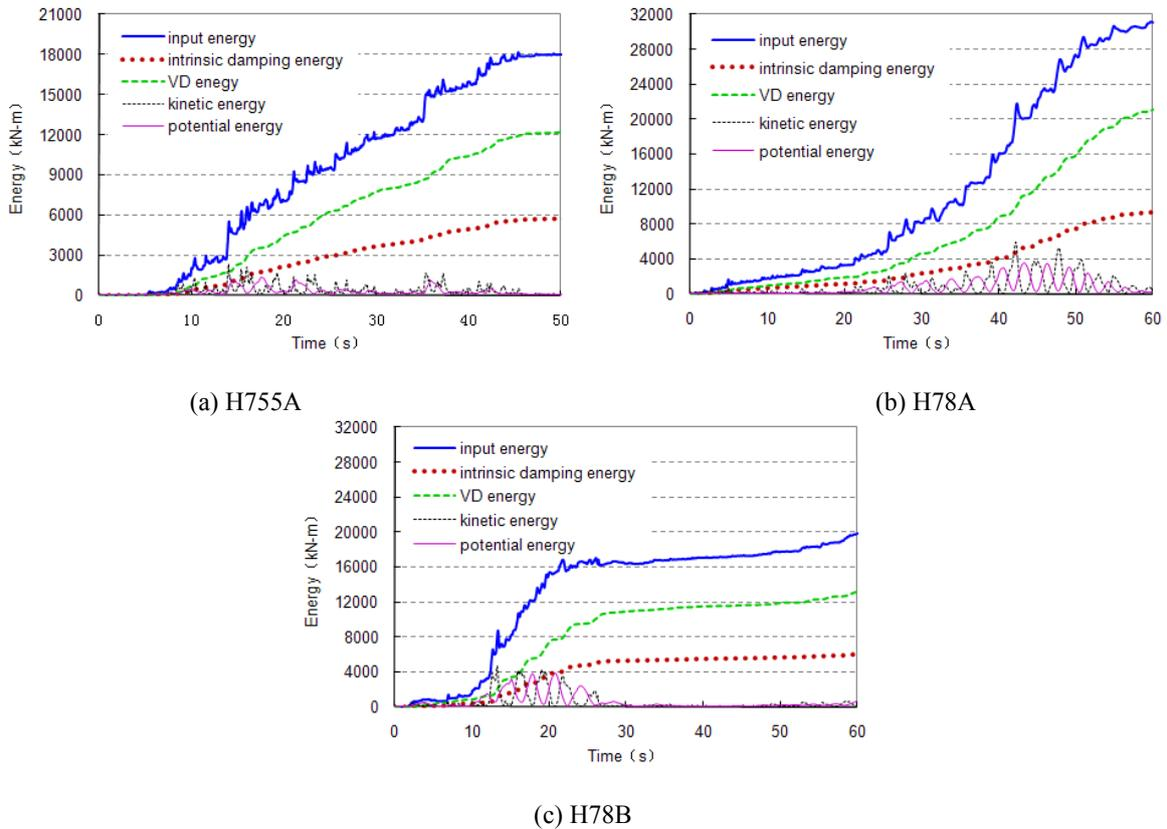
**Figure 4.5** Energy dissipation categories under minor earthquake
