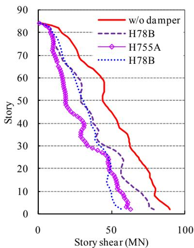
**Figure 4.2** Story shear under minor earthquake
