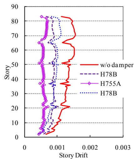
**Figure 4.4** Story drift under minor earthquake
