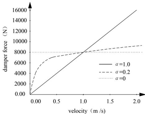
**Figure 2.2** Relationship of damper force and velocity
