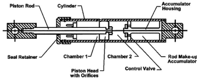
**Figure 2.1** Viscous Damper Sketches
