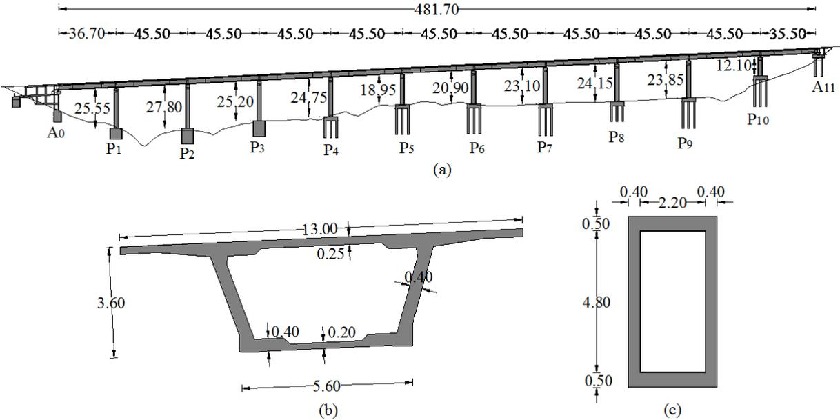
**Figure 3.1.** (a) Longitudinal section of the “reference” bridge, (b) The deck’s cross-section at the mid-span and (c) The pier’s cross-section
