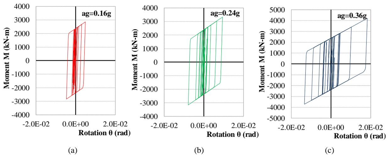
**Figure 3.7.** The hysteresis loops of a wall for design ground acceleration (a) 0.16g, (b) 0.24g and (c) 0.36g
