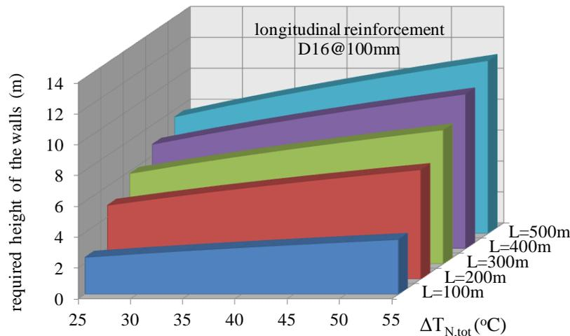
**Figure 3.2.** The minimum height of the walls required by serviceability loading for bridges whose length is 100m, 200m, 300m, 400m and 500m
