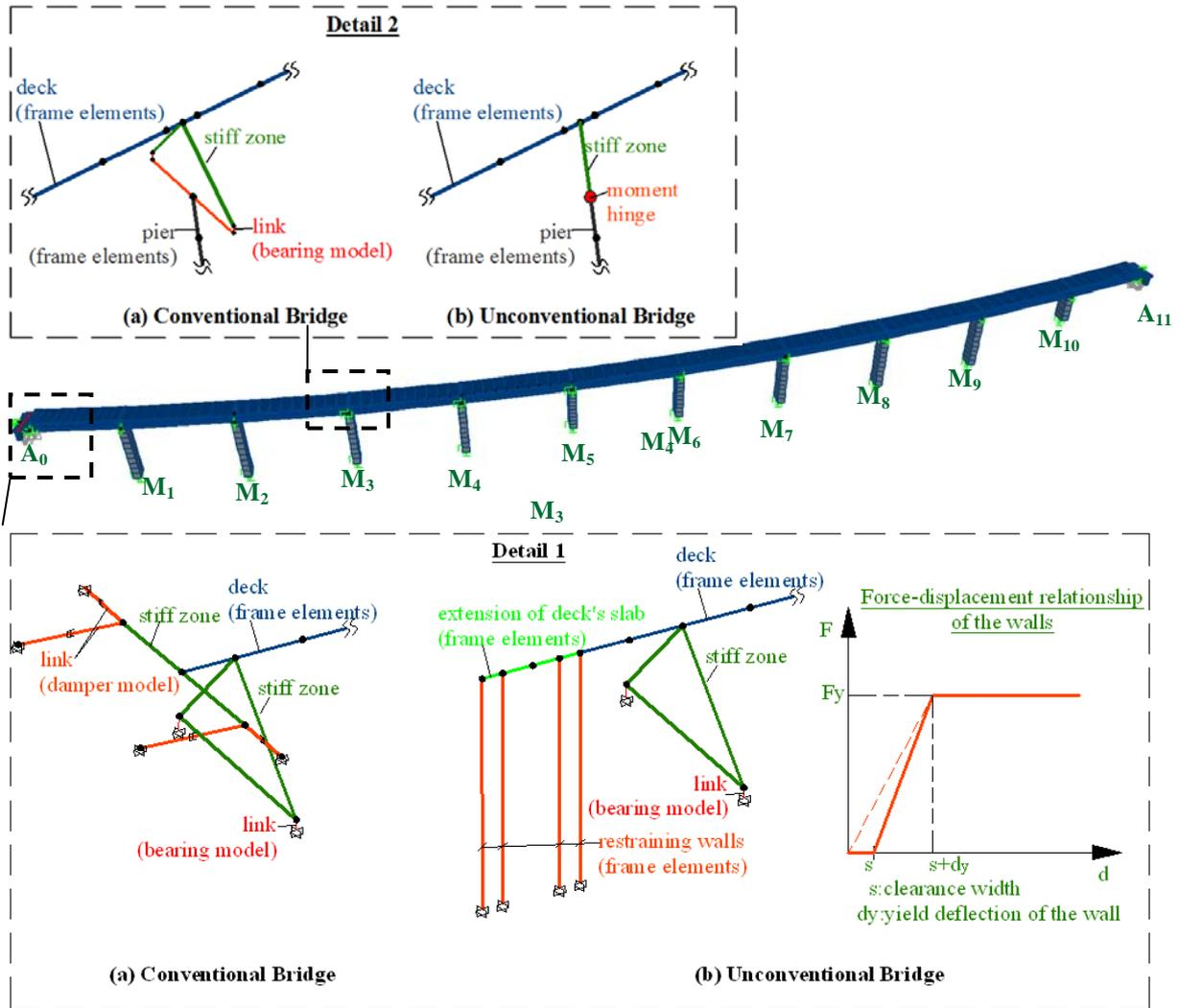
Figure 3.4. The model of the analysed bridge systems
