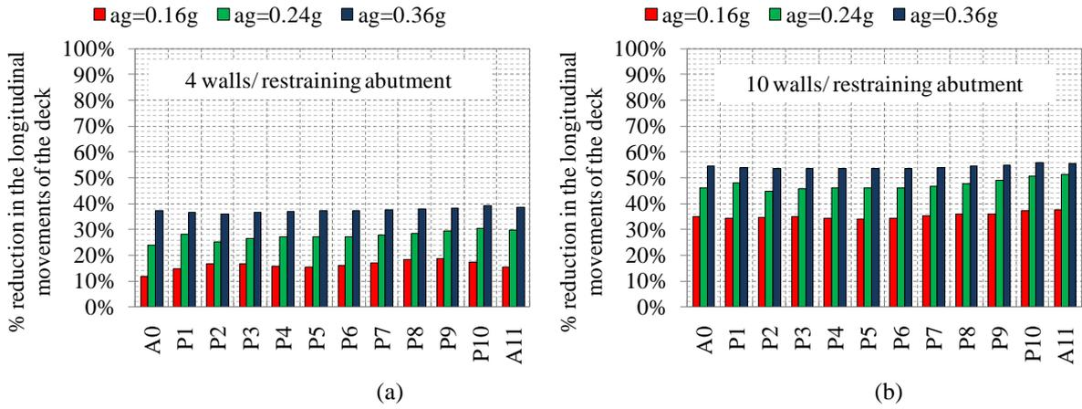
**Figure 3.5.** The percentage reductions in the longitudinal movements of the deck for design ground acceleration 0.16g, 0.24g and 0.36g for abutments consisting of (a) 4 and (b) 10 restraining walls
