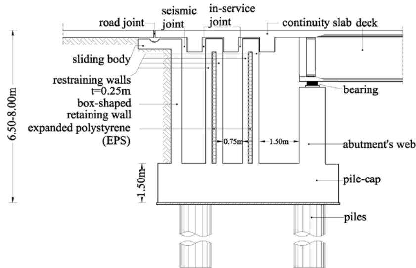
Figure 2.1. Longitudinal section of the proposed abutment
