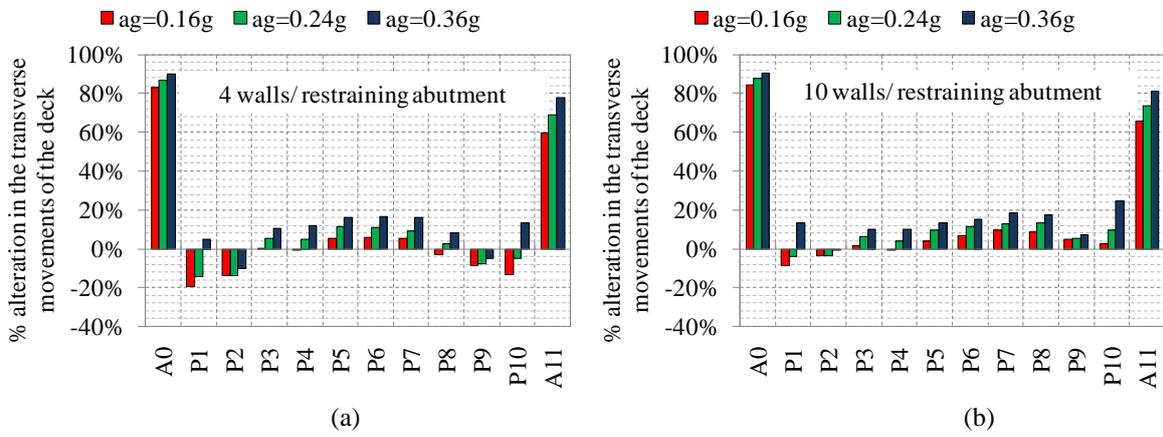
**Figure 3.6.** The percentage alteration in the transverse movements of the deck for design ground acceleration 0.16g, 0.24g and 0.36g for abutments consisting of (a) 4 and (b) 10 restraining walls
