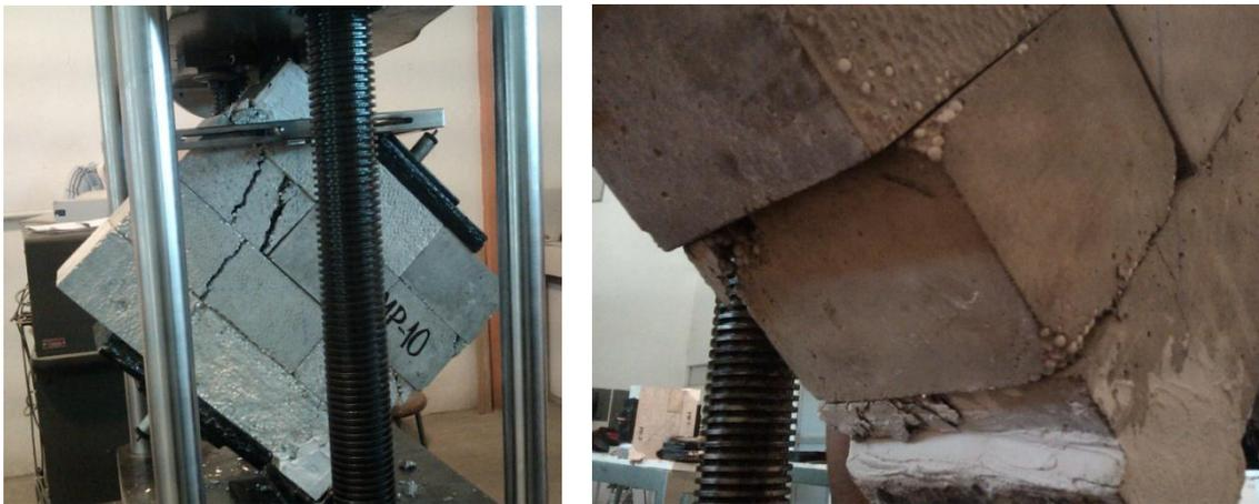
**Figure 4.3.** Cracking and sliding behaviours in a wallet
