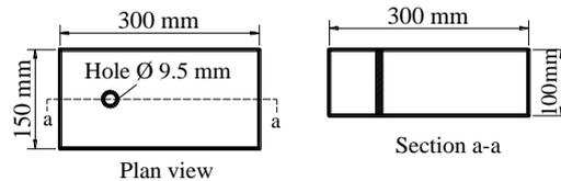
**Figure 3.1.** Masonry piece dimensions
