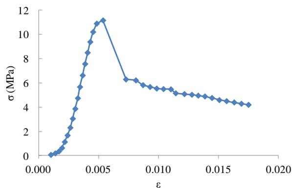
**Figure 4.1.** Stress-strain curve for PCL-7 prism
