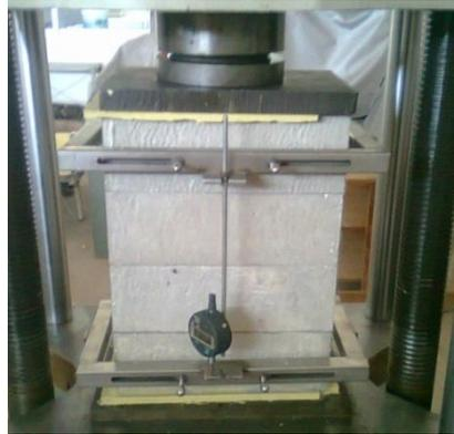
**Figure 3.4.** Masonry prism under testing
