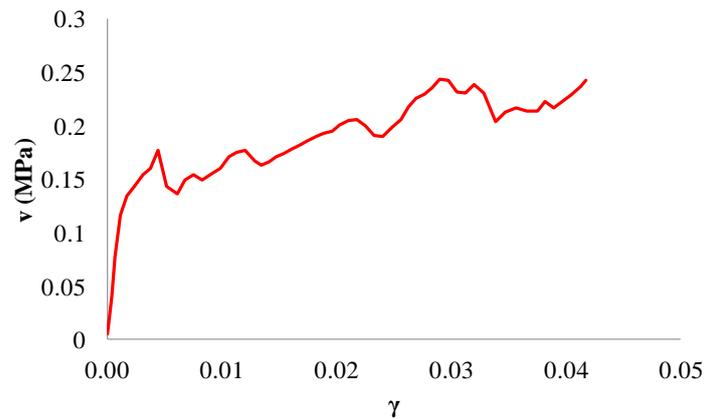
**Figure 4.2.** Shear stress-strain curve for MP-9 wallet
