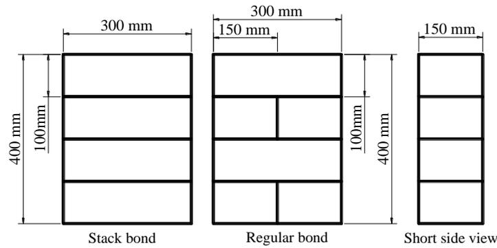
**Figure 3.2.** Masonry prisms dimensions
