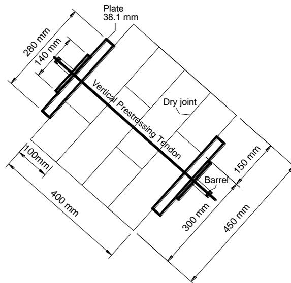
**Figure 3.3.** Masonry wallet dimensions
