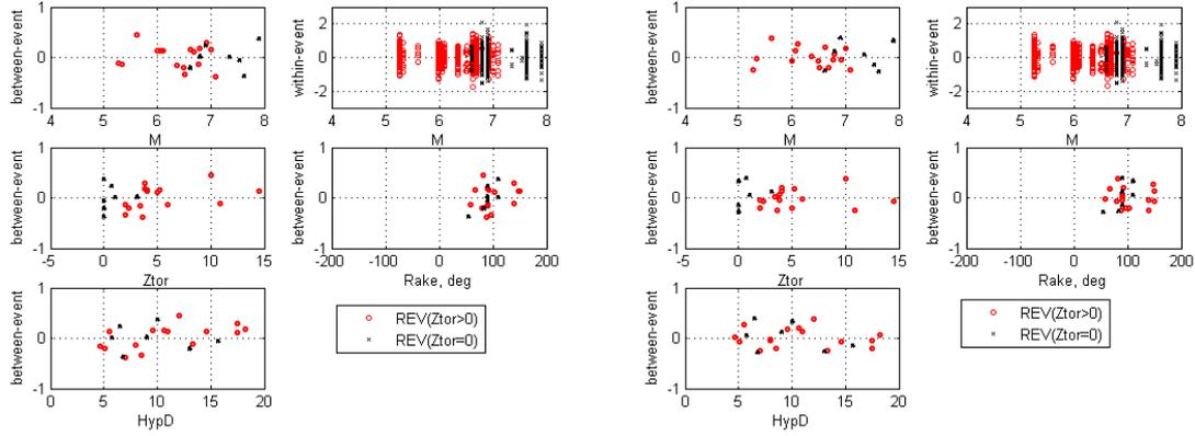
**Figure 3.2.** Inter-event residuals excluding (left) and including (right) the new hypocentral depth term for reverse-faulting mechanisms (smaller black symbols refer to surface-faulting events)
