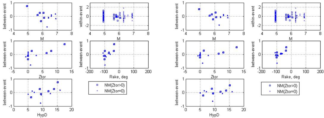
**Figure 3.3.** Inter-event residuals excluding (left) and including (right) the new hypocentral depth term for normal-faulting mechanisms (smaller symbols refer to surface-faulting events)
