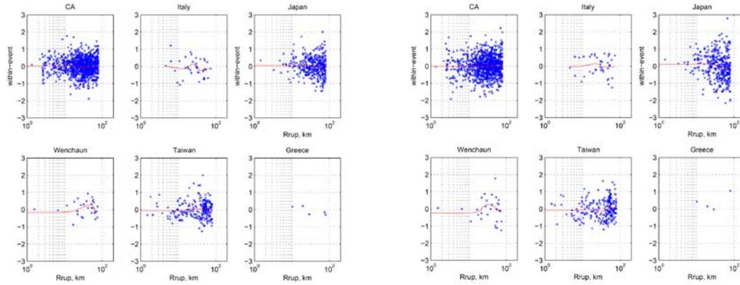
**Figure 4.1.** Intra-event residuals from a GMPE developed for PGA (left) and 1.0-s PSA (right) from recordings obtained within 80 km of the fault rupture plane showing no apparent regional dependence of geometric attenuation
