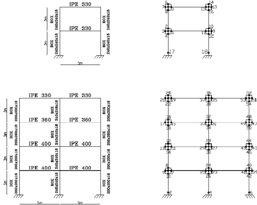
**Figure 1.** Modeling details of the sample frame structures.
