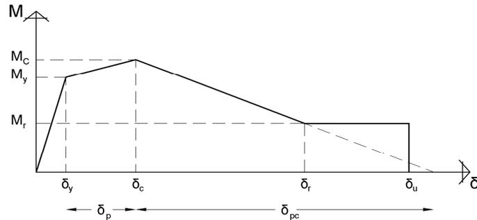
**Figure 2.** Backbone curve of the modified Ibarra-Krawinkler material for element ends.
