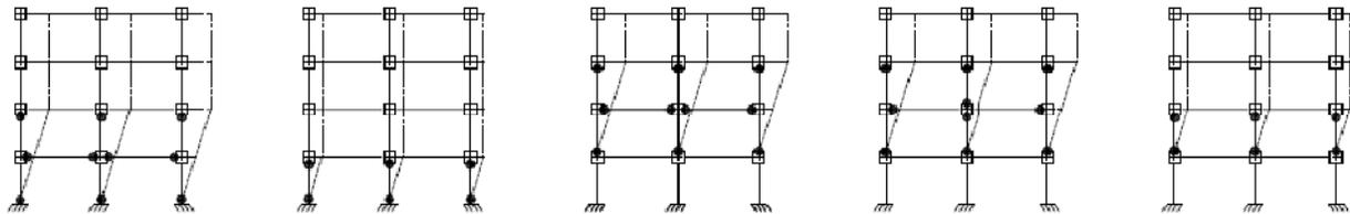
Figure 8. Basic collapse mechanisms of the case study ISMRF
