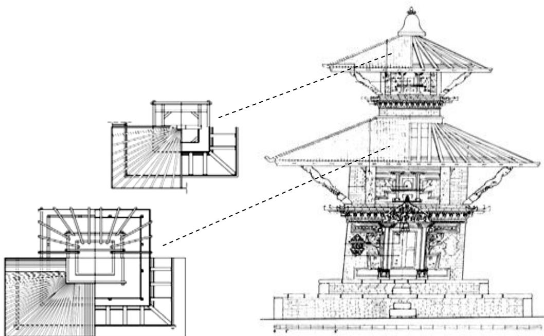
**Figure 2.** Roof construction system in Temples ([Theophile *et al.*, 1992]; [Bonapace *et al.*, 2003])
