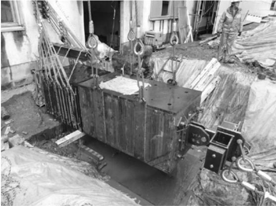
Figure 4. Rubber and Steel mass for impact loading
