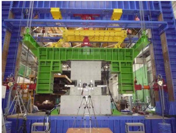
**Figure 9.** The lateral loading test of the placing concrete joint in the laboratory
