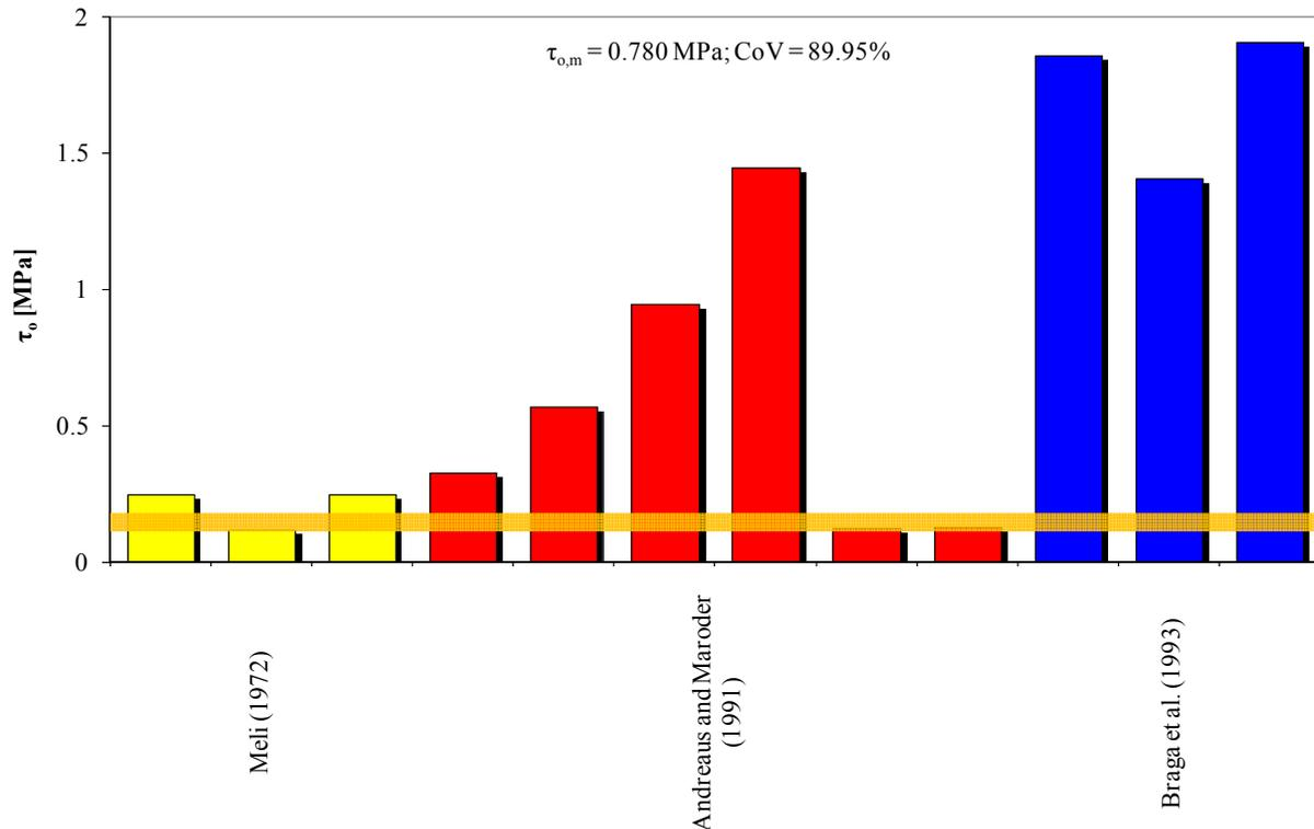
**Figure 4.** Experimental data on shear strength at zero confining stress of brick masonry class 2
