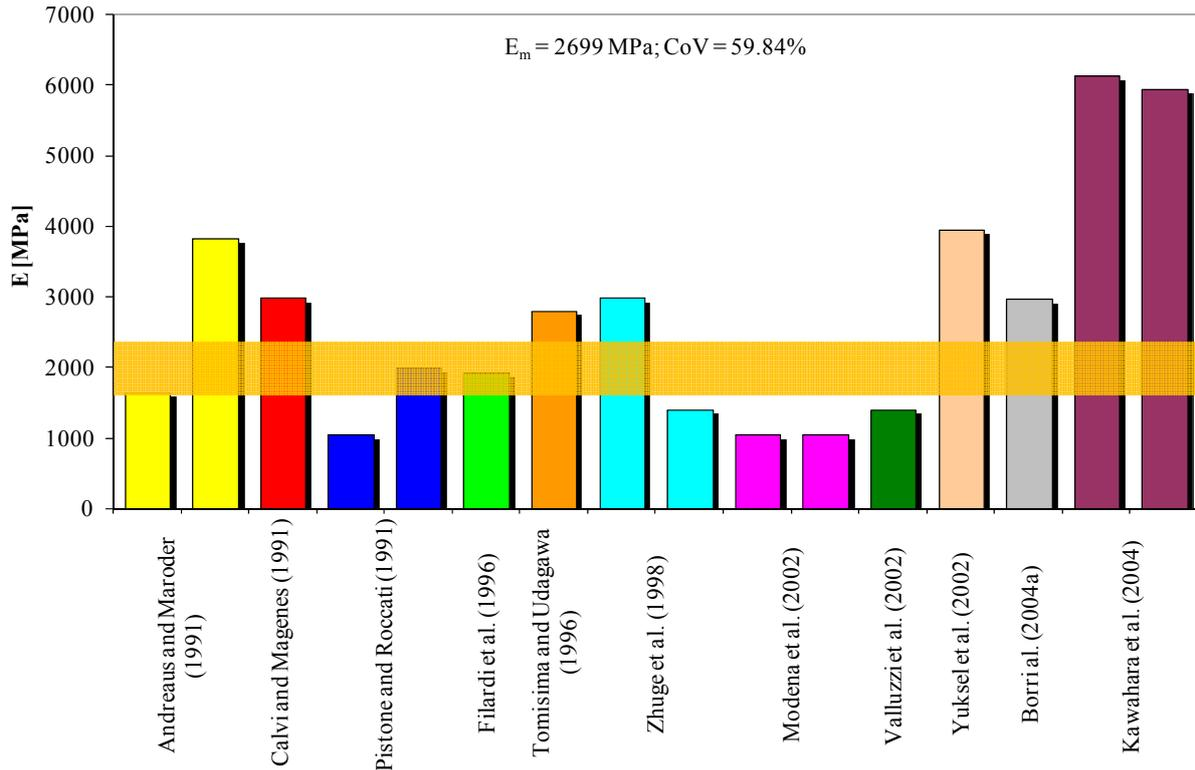
**Figure 5.** Experimental data on Young's modulus of brick masonry class 1
