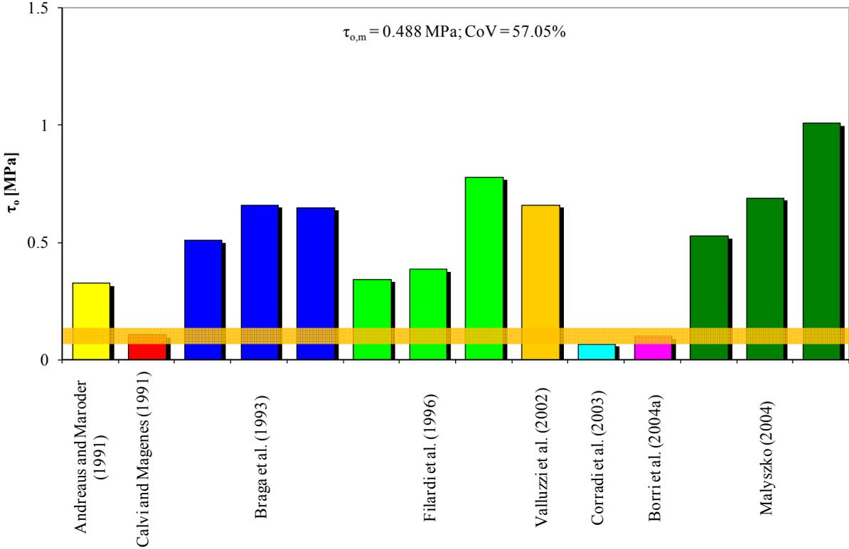
Figure 3. Experimental data on shear strength at zero confining stress of brick masonry class 1
