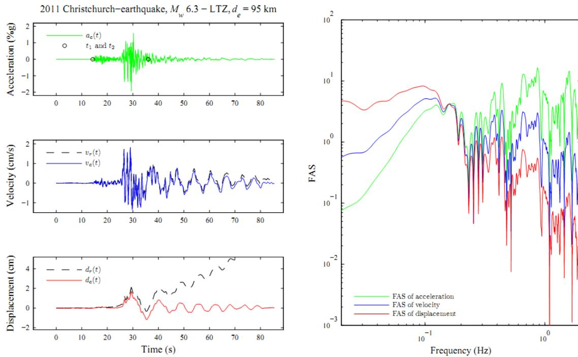
**Figure 7.** The East-component at LTZ-station recorded at the 2011 Christchurch earthquake. Acceleration, velocity and displacement traces (*left*) and corresponding Fourier amplitude spectra (*right*). The raw waveforms are indicated by a dashed line while the baseline adjusted waveforms are plotted with a solid line. The displacement waveform is plotted for filtered data in Fig. 1.
