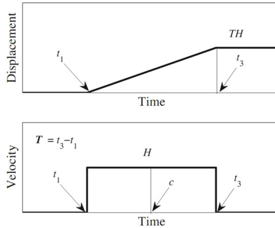
**Figure 3.** Displacement modelled as a ramp (top) and the corresponding velocity (bottom), which is a boxcar of width  $T$  and centred at  $c$ . The displacement starts at  $t_1$  and reaches a maximum value of  $TH$  at time  $t_3$  after which it remains constant. The slope of the ramp is equal to the height of the boxcar.
