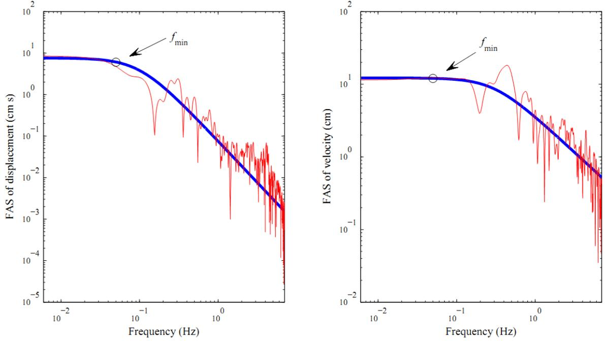
**Figure 4.** Fourier amplitude spectra (FAS) of two records from the May 2008  $M_w$  6.3 Ölfus earthquake. *Left:* Displacement-FAS of Hella-record at an epicentral distance of 36 km (red curve) and the corresponding Brune far-fault spectrum (blue curve). *Right:* Velocity-FAS of Selfoss-Hospital-record at an epicentral distance of 8 km (red curve) and the corresponding Brune near-fault spectrum (blue curve). The records have been processed by the procedure proposed in the present paper.
