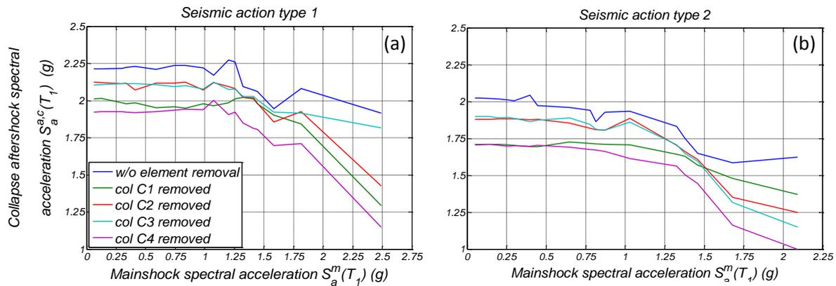
**Figure 4.4.** Mean aftershock spectral acceleration that leads the structure to collapse as a function of the mainshock spectral acceleration for: (a) seismic action type 1; and (b) seismic action type 2
