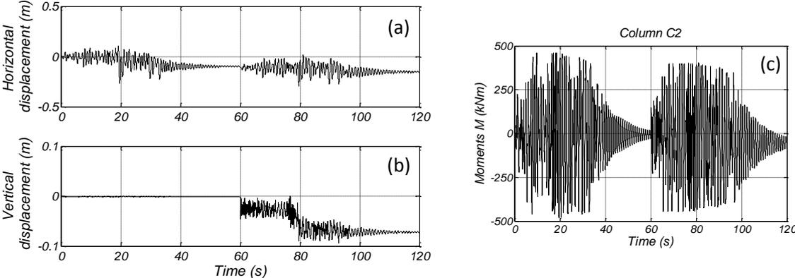
**Figure 4.3.** (a) Roof horizontal displacement above column C1; (b) Roof vertical displacement above column C1; and (c) Bending moments at base of column C2
