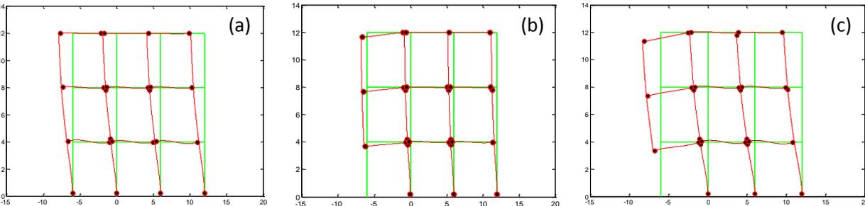
**Figure 4.2.** Deformed shape of the structure at instants when: (a) peak roof displacement during the mainshock is achieved; (b) 1s after the column C1 has been removed; and (c) maximum roof displacement during the aftershock
