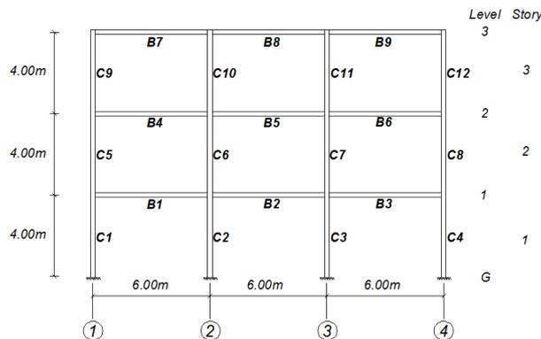
Figure 4.1. Steel Moment Resisting Frame
