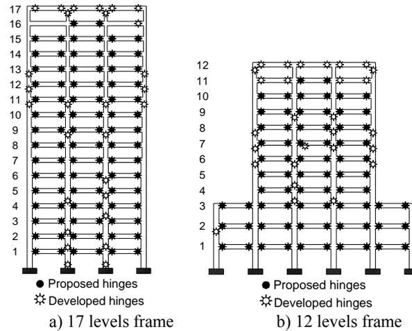
**Figure 6.2.** Comparison of the damage distribution expected with that produced by the design earthquake associated with the CPLS
