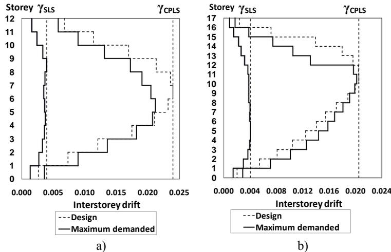
**Figure 6.1.** Comparison of the design interstorey drifts with the maximum demanded for a.) 12 levels frame and b.) 17 levels frame
