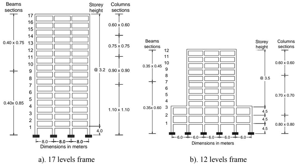
**Figure 5.1.** Geometric configurations of the two example frames
