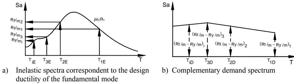
**Figure 2.2.** Design seismic demands
