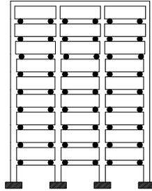
**Figure 4.1.** Potential distribution of damage consistent with the collapse prevention limit state
