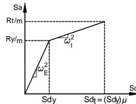
**Figure 2.1.** Behaviour curve of a SDOF bilinear oscillator
