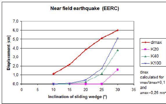
(a) Near field motion  $v_{max}/a_{max}=0.1$ ;  $a_{max}=0.26 \text{ m/s}^2$
