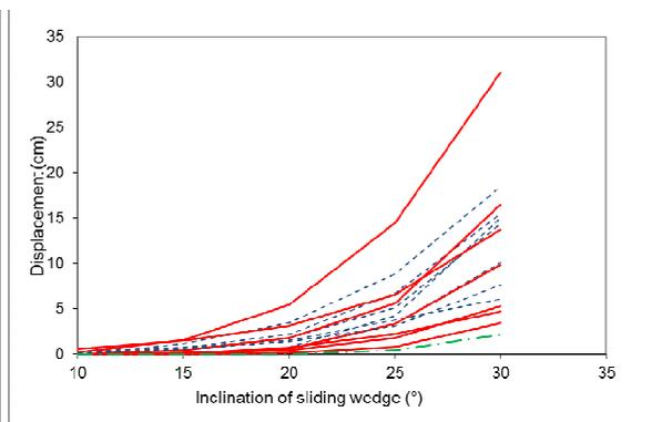
b) Revised seismic criteria considering 70 m high dam model (Solid line and dashed line: results for the normal faulting earthquake of magnitude 6.2 and 6.0 respectively; Dash-dotted line: results for the strike slip earthquake of magnitude 5.3)
