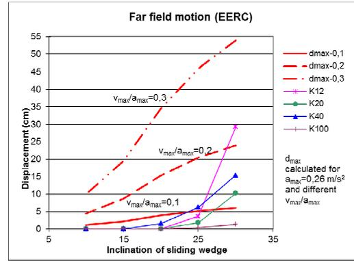
(b) Far field motion  $v_{max}/a_{max}=0.1, 0.2$  and  $0.3$  (labelled  $d_{max-0.1}, d_{max-0.2}$  and  $d_{max-0.3}$  respectively) and with  $a_{max}=0.26 \text{ m/s}^2$
