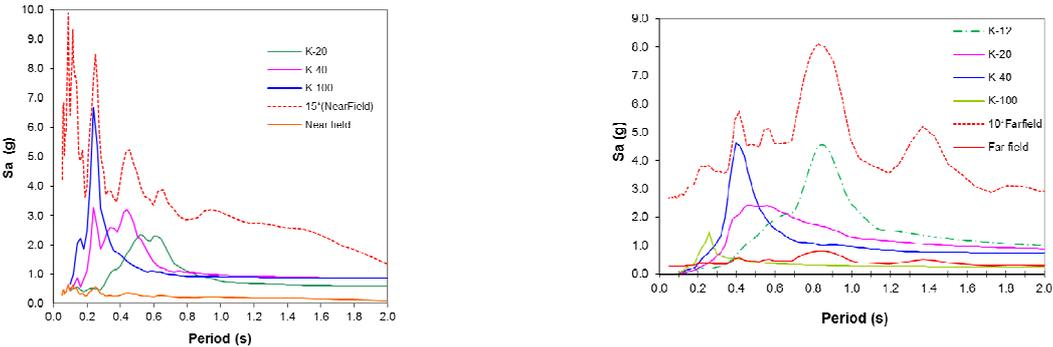
(a) Near field motion with  $a_{max}=0.26$  g. The data series labelled 15\*(Near Field) is the spectral ordinates of the input motion scaled 15 times.
