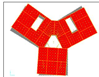
**Figure 2.4.** First vibration mode    **Figure 2.5.** Second vibration mode    **Figure 2.6.** Third vibration mode
