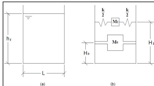
**Figure 3.1.** Circular TLD: (a) real prototype at rest, (b) equivalent mechanical model [Newmark and Rosenblueth, 1971]
