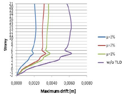
Figure 6.2. Drift profile envelope
