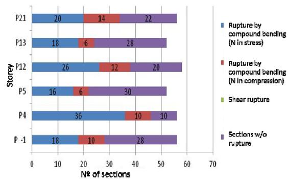
**Figure 19.** Ratio of sections that match the limits of rupture and the conditions of safety for seismic loads (with TLD)
