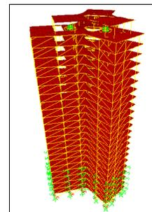
**Figure 4.2.** Disposal of TLD's in the mechanical model
