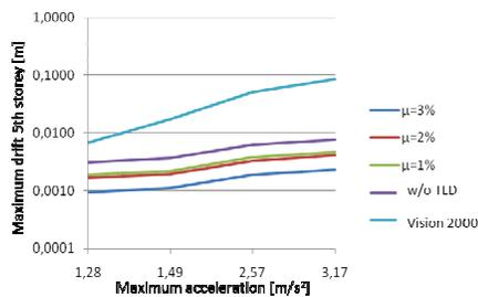
Figure 6.3. Maximum Lateral Displacement for each structure and return period (5<sup>th</sup> floor)
