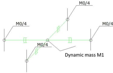
**Figure 3.2.** Macro-model of a TLD implemented in commercial program SAP2000NL [SAP2000NL, 2003]
