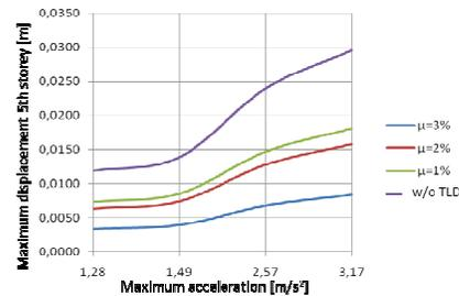
Figure 6.4. Maximum drift requirement for each structure and return period (5<sup>th</sup> floor)
