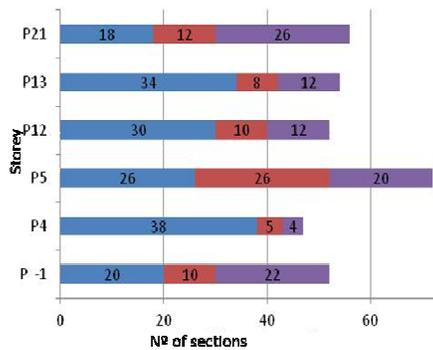
**Figure 18.** Ratio of sections that match the limits of rupture and the conditions of safety for seismic loads (without TLD)
