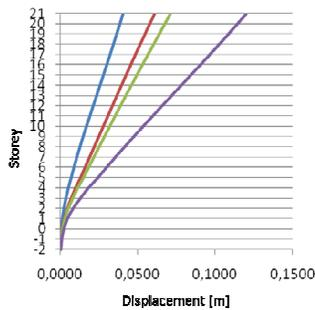
Figure 6.1. Lateral displacement envelope
