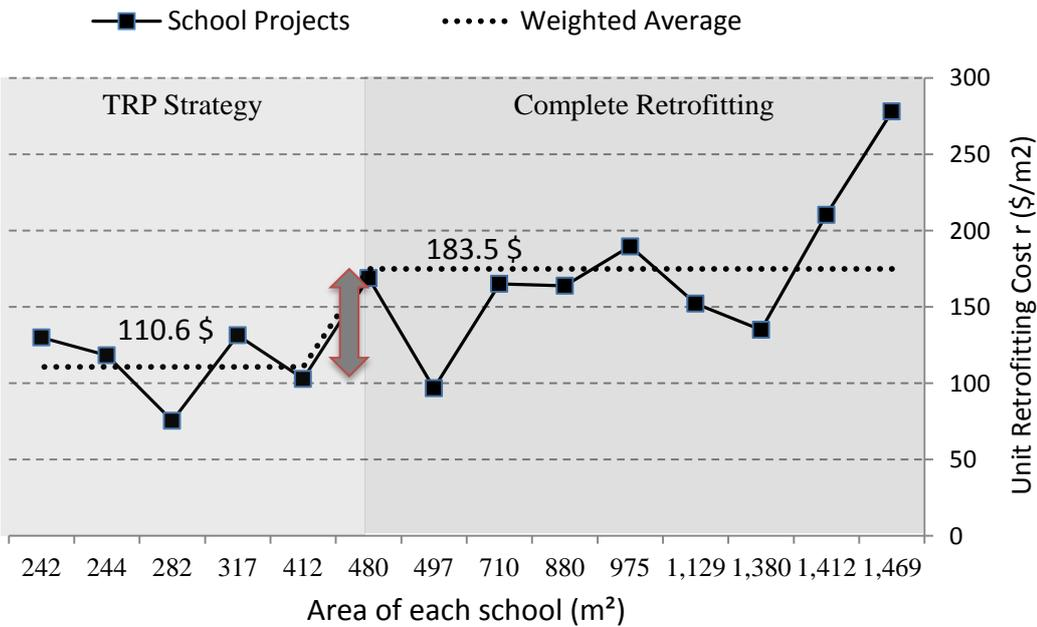
**Figure1.** Final cost of retrofitting per square meter with respect to square of each school for complete retrofitting and TRP approaches
