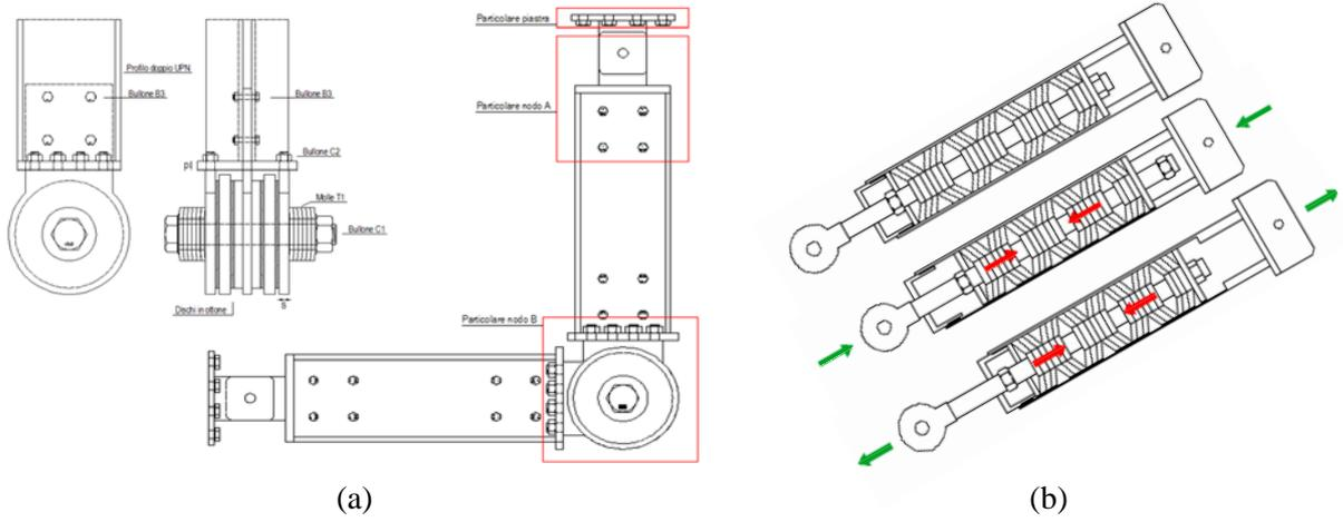
**Figure 3.1** Details of the device dissipating energy by friction made of one disk with 4 rotating surfaces (left) and diagonal elastic spring devices (right).
