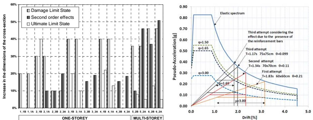
**Figure 2.1** New designed structures with pinned beams and monolithic columns: increment of the section of the column to limit the second order effects and the excessive displacements at the damage limit state (left); stiffness increment and subsequent reduction of the behaviour factor  $q$  (from 3 to 1.65 in the case depicted in figure) necessary to limit the second order effects (right).
