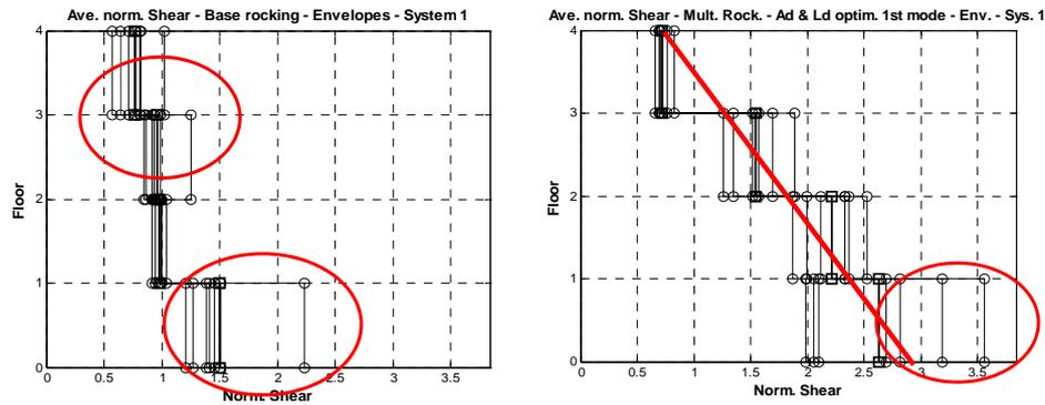
**Figure 6.3** Four-storey buildings: normalized shear distribution for base rocking (left) and for dissipaters optimized for first mode of vibration (right).
