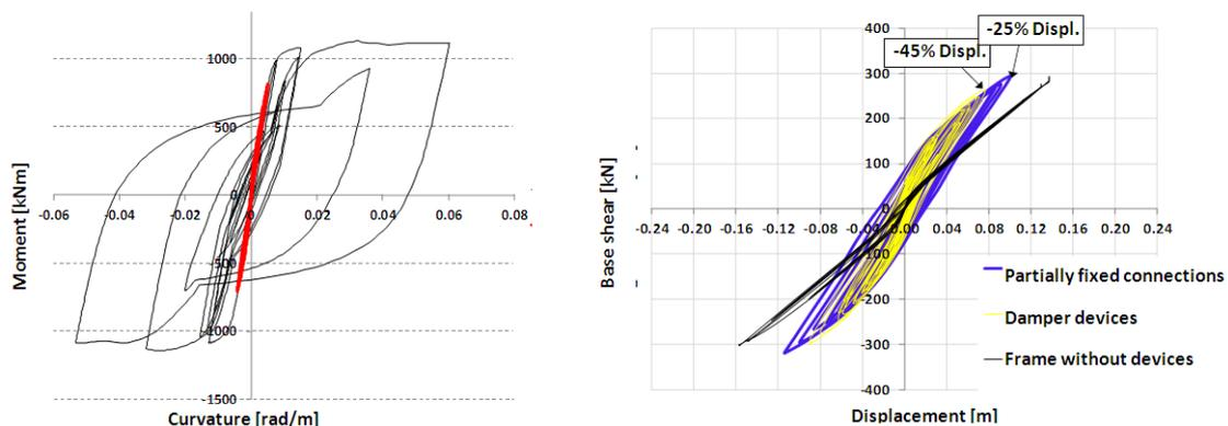
**Figure 3.4** Moment-Curvature at the base of a one-storey structure with and without friction devices (red and black lines, left) and top displacement vs. base shear curves of one-storey structure with and without devices (black line: hinged frame; blue line: partially fixed connections; yellow line: viscous dampers, right).
