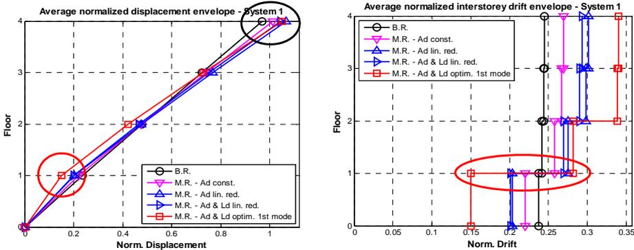
**Figure 6.1** Four-storey buildings: average value of the normalized displacement (left) and drift (right).
