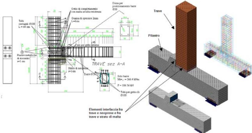
**Figure 4.1** Details of the specimen (left) and finite element model developed to evaluate the numerical prediction of the cyclic response of the system of connection (right).
