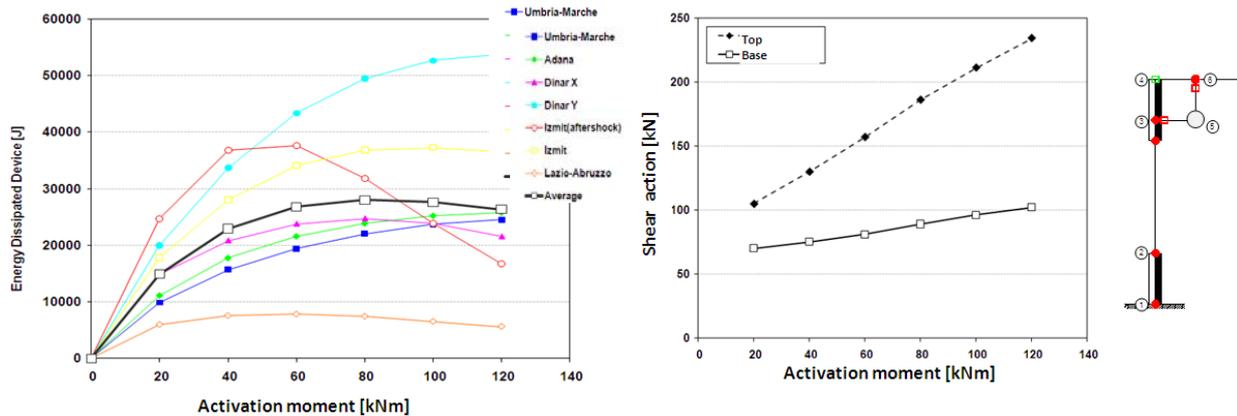
**Figure 3.3** Friction devices: energy dissipated by the device as a function of the moment of activation (the average values are depicted with the black line, left) and top and base shear on the column (right).
