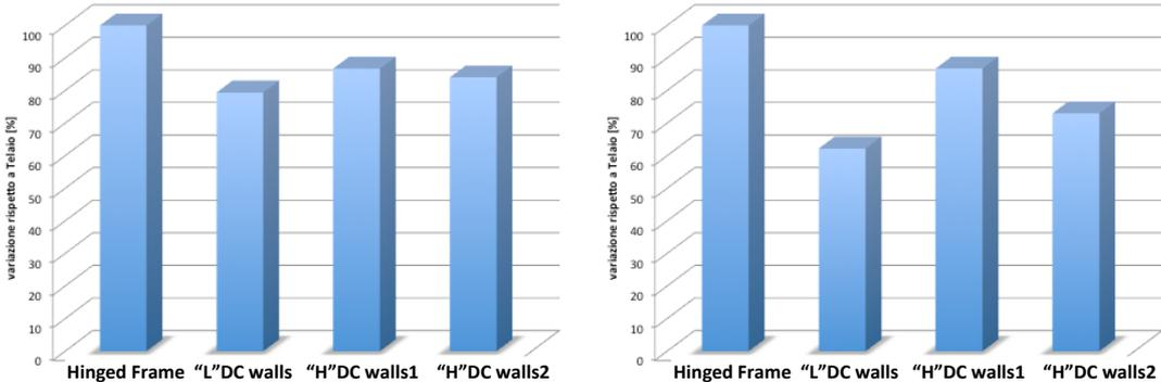
**Figure 5.1** Comparisons in terms of amount of concrete (left) and steel bars(right) of the examined case-studies: from the left to the right: hinged frame, perimeter walls calculated in low ductility class, two different perimeter walls distributions calculated in high ductility class (right).
