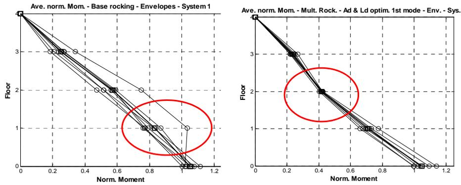
**Figure 6.2** Four-storey buildings: normalized moment distribution for base rocking (left) and for dissipaters optimized for first mode of vibration (right).
