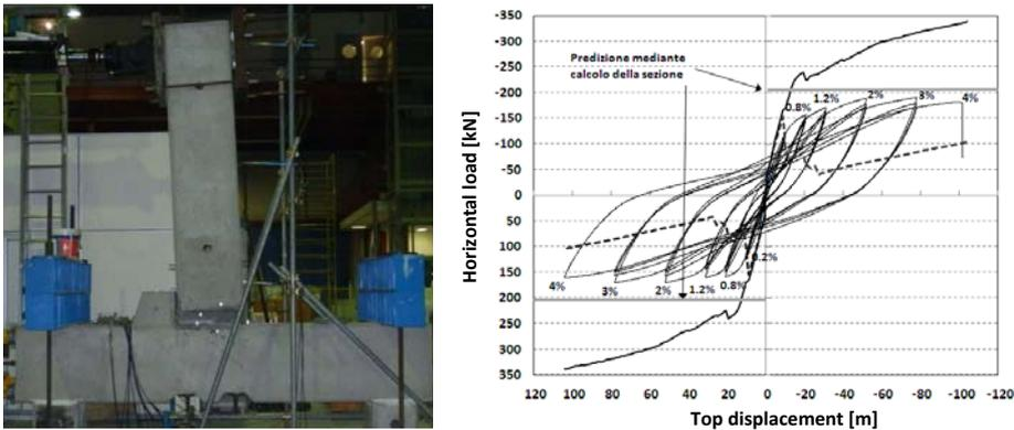
**Figure 4.2** Experimental tests: deformed configuration at 3% of drift level (left) and experimental force vs. displacement curves compared to numerical predictions developed under different hypotheses (right).
