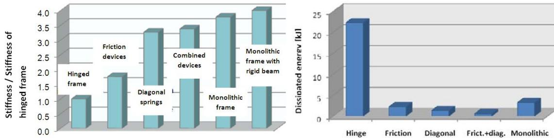
**Figure 3.2** Stiffness of the system (left) and energy dissipated by the column (right) as a function of the typology of considered device.
