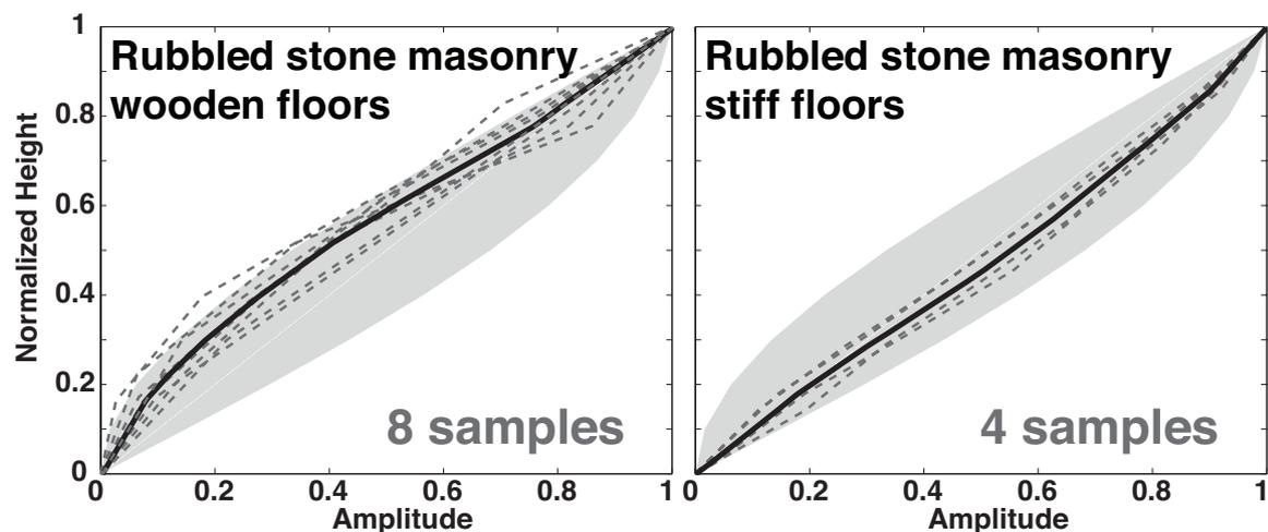
**Figure 1.** Modal shape of the fundamental mode for stone masonry structures with wooden and stiff floors. Black thick line is the average of the class. Grey zone represents the theoretically possible range of behaviour.
