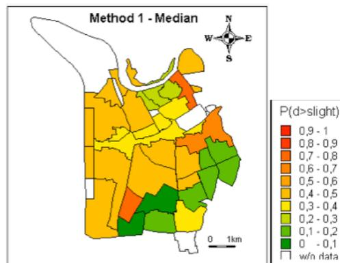
**Figure 3.** Damage distribution in the city of Grenoble: rate of structures exceeding the slight damage state in each zone.
