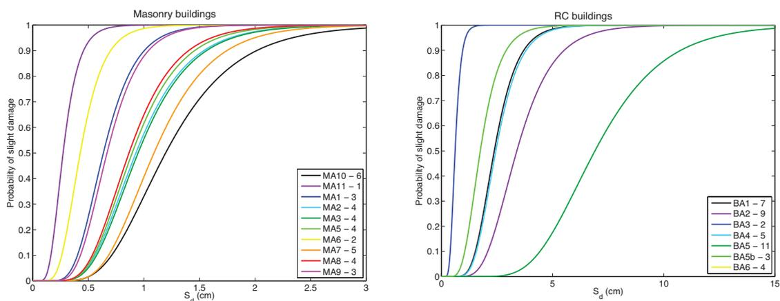
**Figure 2.** Fragility curves for slight damage for the different building classes in Grenoble
