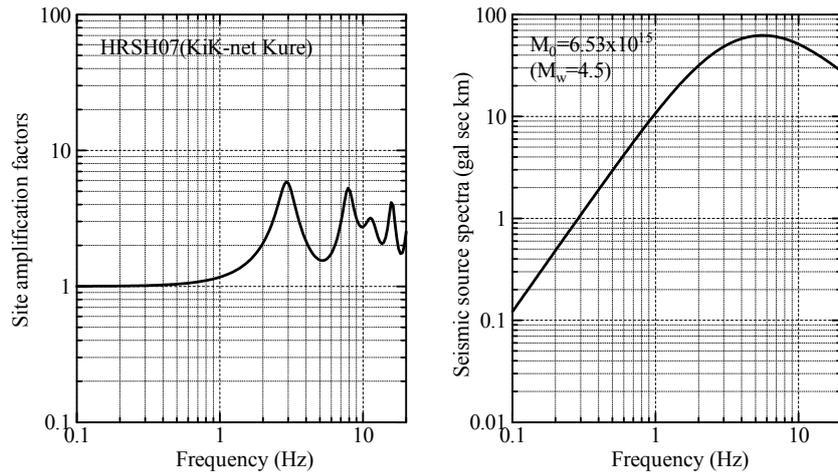
Figure 3.1. Theoretical site amplification characteristics (left figure).
