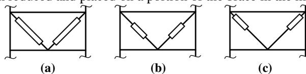
**Figure 2.** Normal length and reduced length BRBs with different core positions
