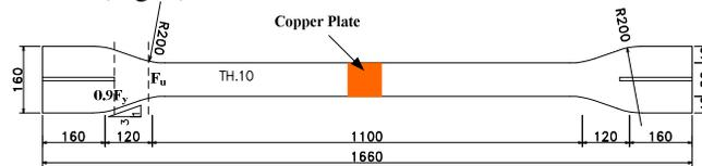
Figure 8. Plan of BRB core with copper plate
