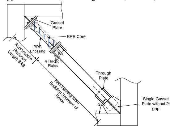
Figure 1. Reduced length BRB in a frame
