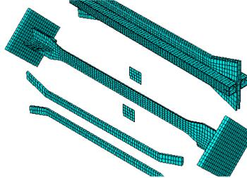
Figure 13. Finite element model of proposed BRB
