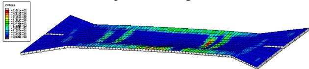
**Figure 16.** Deformed shape and normal contact force on encasing at maximum compressive displacement
