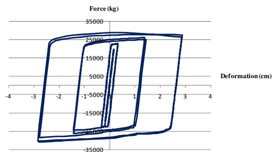
Figure 14. Finite element analysis result for RLBRB
