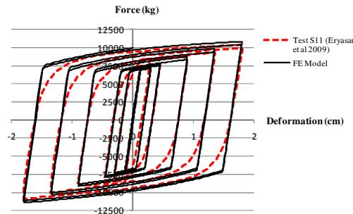
**Figure 11.** Finite element analysis and test results for specimen 11
