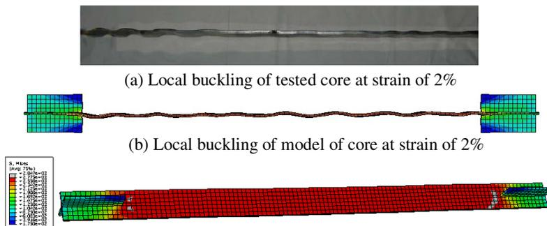
**Figure 12.** Deformation and stress state of specimen 11
