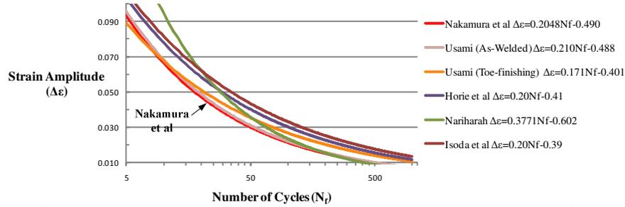
**Figure 4.** Coffin Manson Equations developed based on experimental results
