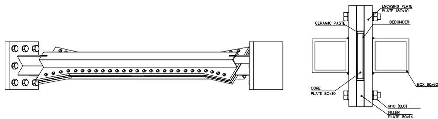
**Figure 7.** 3D view and section of RLBRB
