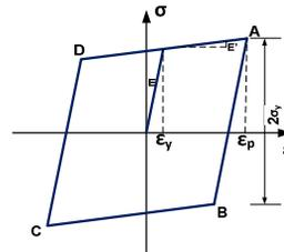
**Figure 6.** Stress strain hysteresis loop for BRB
