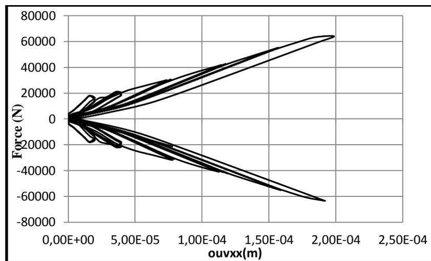
**Figure 5.7** The evolution of the axial crack openings under cyclic loadings (Forces Vs Crack Openings)
