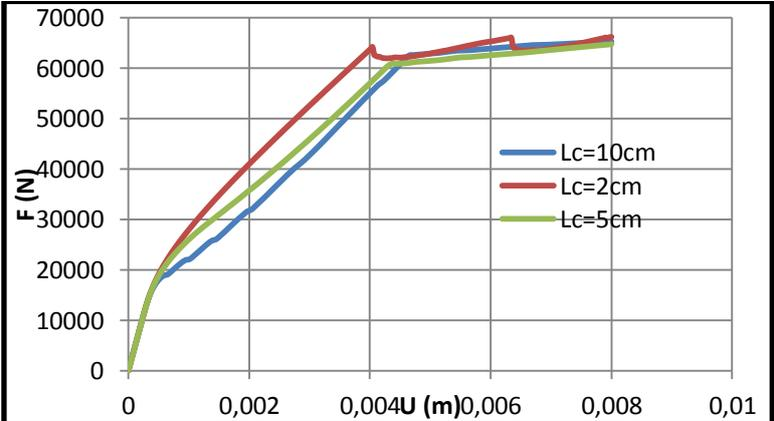
Figure 5.3 The Global response of the LMT beam under static monotonic loading.
