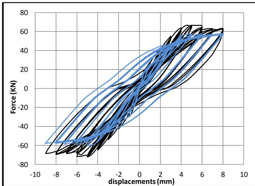
Figure 5.5 Comparison Model-Test responses (Test 2)
