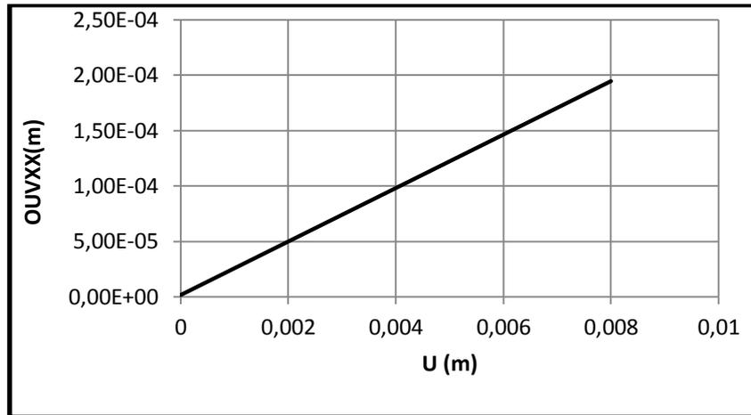
**Figure 5.6** The evolution of the axial crack openings under monotonic static loadings (Crack openings Vs Imposed displacements)
