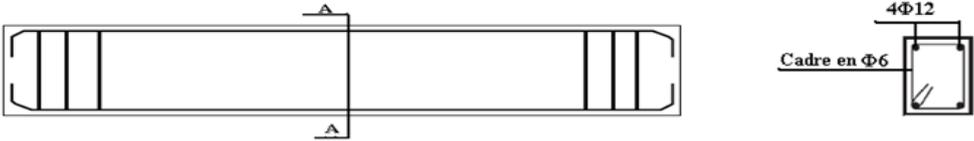
Figure 5.1 The longitudinal and transverse reinforcements of the LMT beam.
