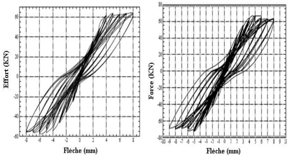
Figure 1.4 The experimental global behavior response a-Test1 b-Test2
