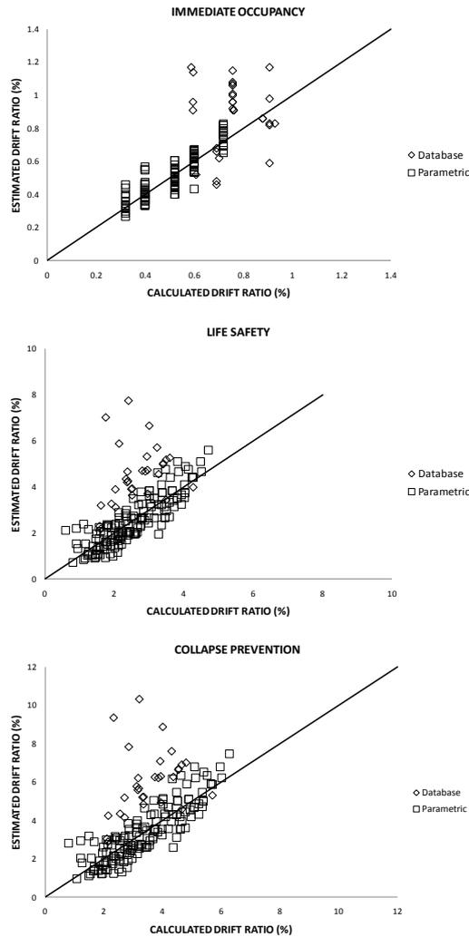
**Figure 4-2** Comparison of Estimated and Calculated Drift Ratios
