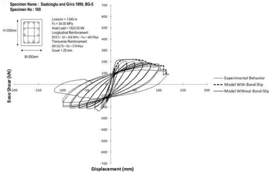
**Figure 3.1.** Effect of Modeling Bond-Slip on Envelope Response
