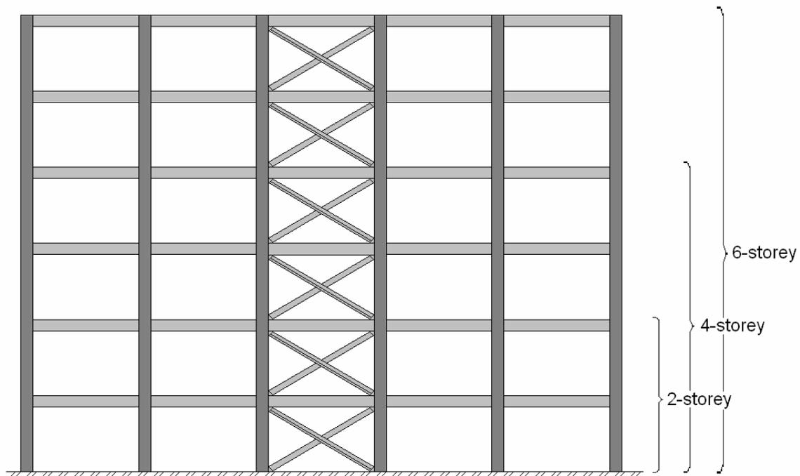
**Figure 2.** Vertical layout of the three buildings
