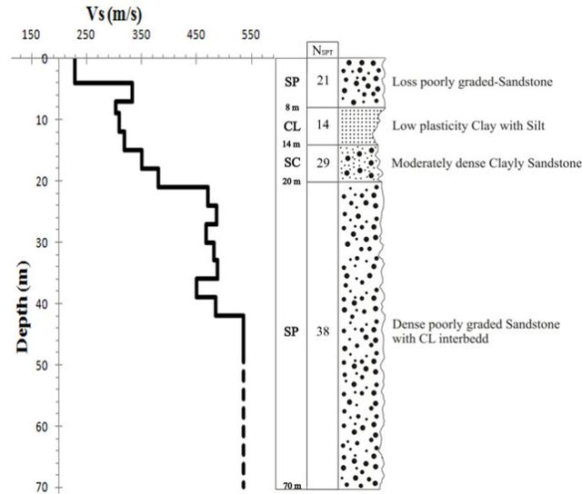
**Figure 2.2.** Geological column gained by direct drilling and sampling with 70m depth along with SPT test results and shear wave velocity profile obtained from downhole test
