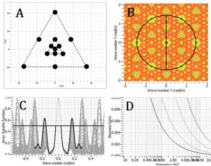
**Figure 3.2.** The general figure of the array configuration and the location of receivers (A), the theoretical response for array A with 13 receivers in  $(K_x, K_y)$  space (B), the transfer functions for different propagation directions (C) and  $K_{Max}$  and  $K_{Min}$  values in frequency-slowness domain (D)
