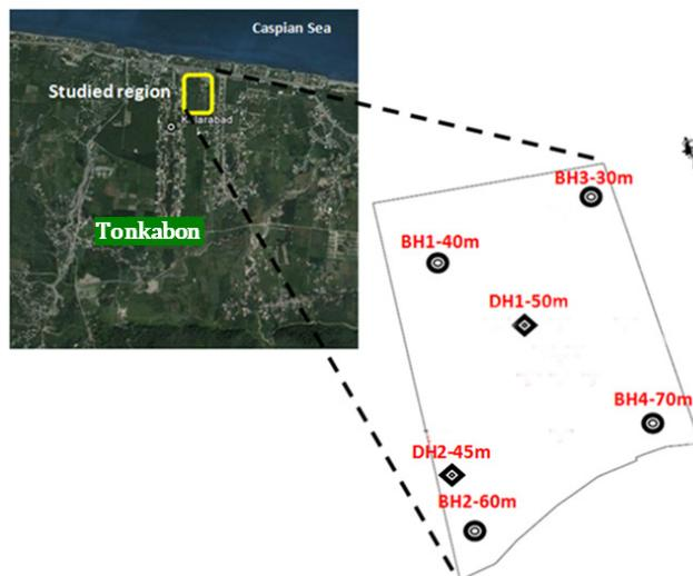
**Figure 2.1.** Aerial photo of studied area along with the location of geotechnical /geophysical boreholes (BH=geotechnical borehole and DH=geophysical borehole)
