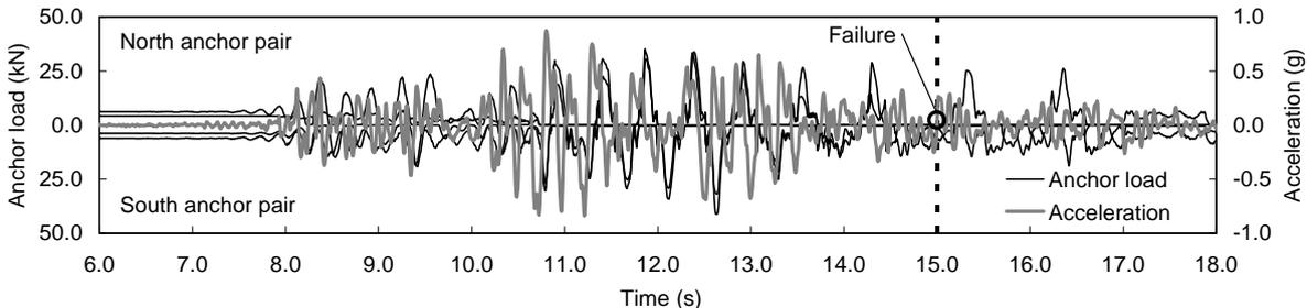
Figure 3.4. Anchor load and acceleration time histories for final failure test on expansion anchors (60 % scaling)
