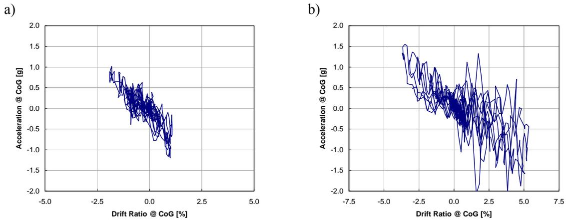
**Figure 3.7.** Acceleration versus drift ratio of the model component for the final failure tests on a) undercut anchor and b) expansion anchor
