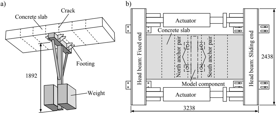
**Figure 2.3.** a) Isometric view of model component connected to concrete slab; b) Plan view of loading rig with mounted concrete slab (all units in mm)
