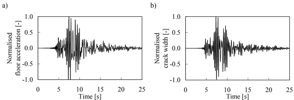
**Figure 2.4.** Normalised time histories for a) floor acceleration and b) crack width
