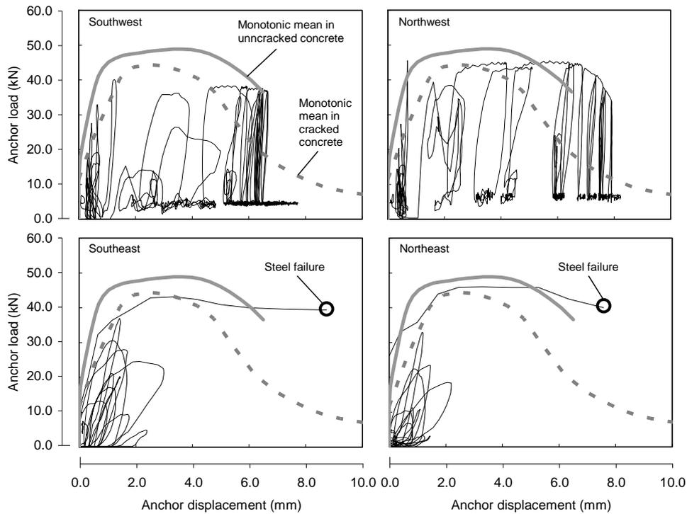
**Figure 3.5.** Load-displacement curves of final failure test on the undercut anchor (130 % scaling)
