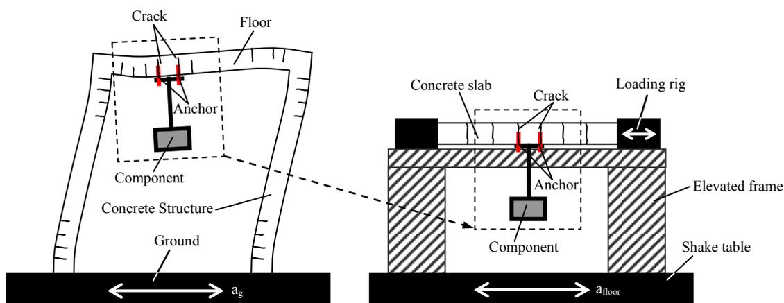
**Figure 2.1.** Component connected to real structure (left) and to model concrete component mounted in loading rig on shake table (right)
