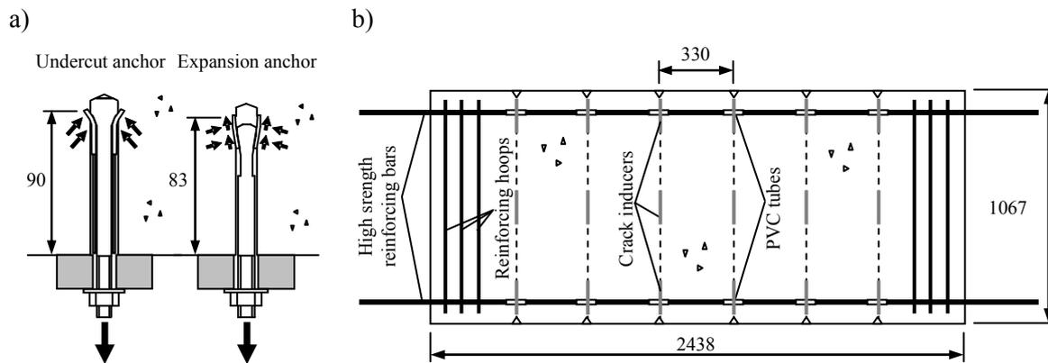
**Figure 2.5.** a) Post-installed anchor types considered in this study; b) Geometry, reinforcement and details of model concrete slabs (all units in mm)
