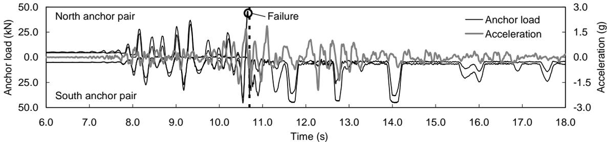
Figure 3.3. Anchor load and acceleration time histories for final failure test on undercut anchors (130 % scaling)
