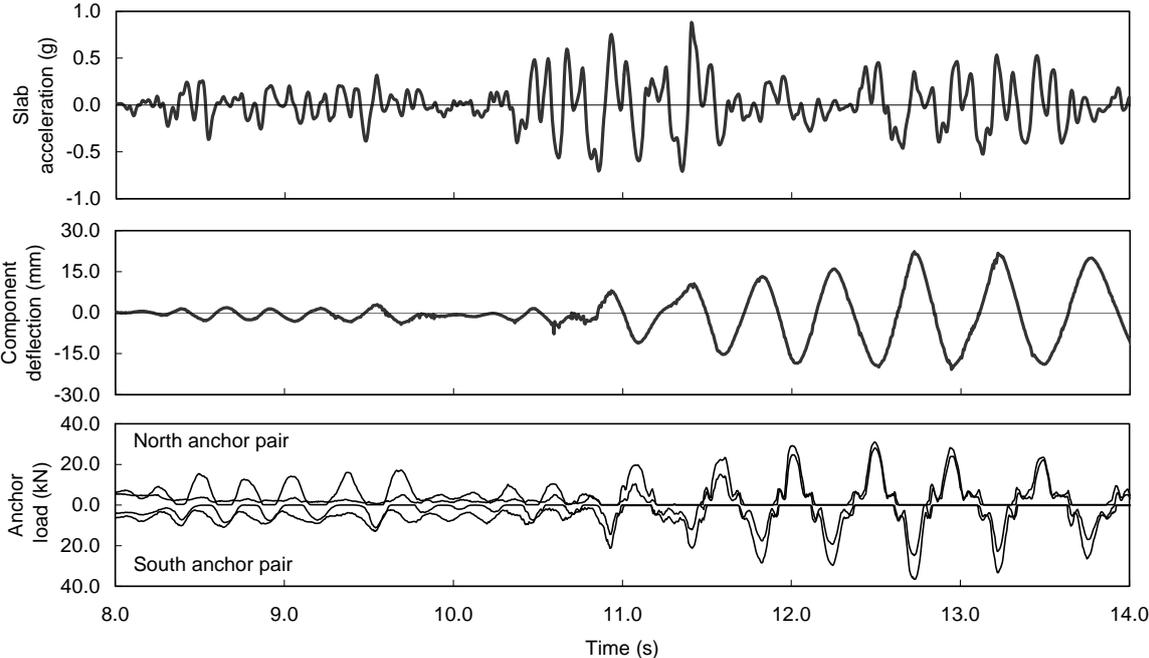
**Figure 3.2.** Time histories of floor acceleration, component deflection and anchor loads (example: Undercut anchor, 40% scaling)
