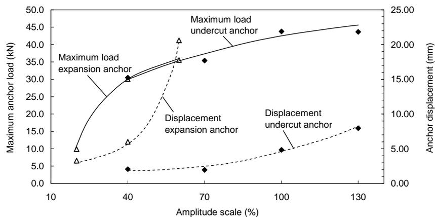
**Figure 3.8.** Maximum anchor load and accumulated anchor displacement versus amplitude scales (trend lines are nonlinear regressions)
