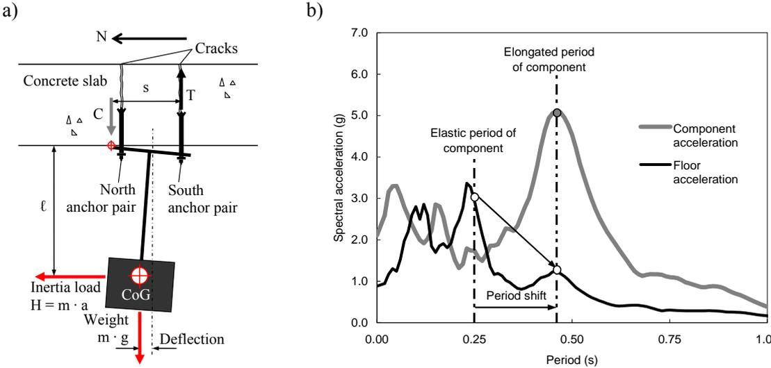
**Figure 3.1.** a) Schematic load transfer mechanism; b) Elastic acceleration spectra of the measured floor and component accelerations (example: Undercut anchor, 40% scaling)
