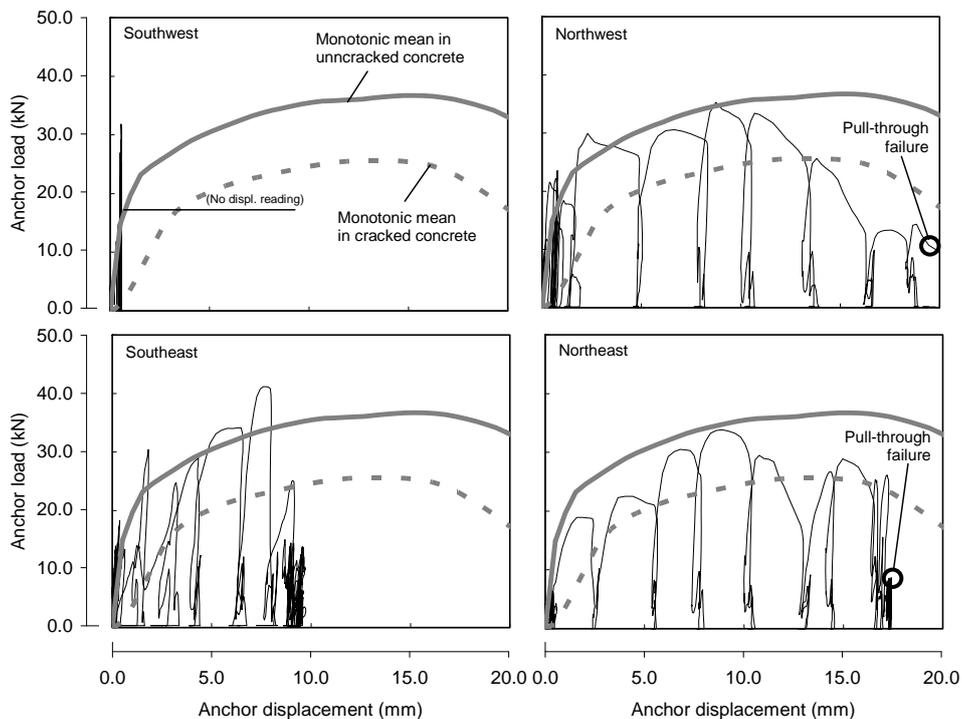
**Figure 3.6.** Load-displacement curves of final failure test on the expansion anchor (60 % scaling)
