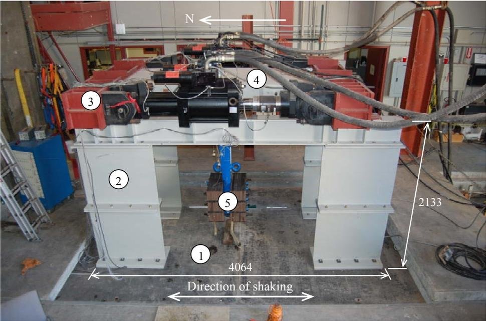
**Figure 2.2.** Picture of test setup (all units in mm)
